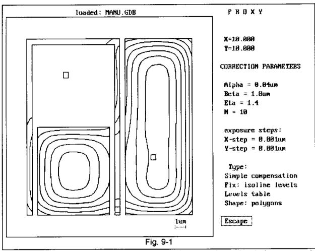
Fig. 9-1 shows a structure, which needs proximity correction at least when exposed on GaAs. Gates, gaps, dot and hole are 0.5 µm wide.
