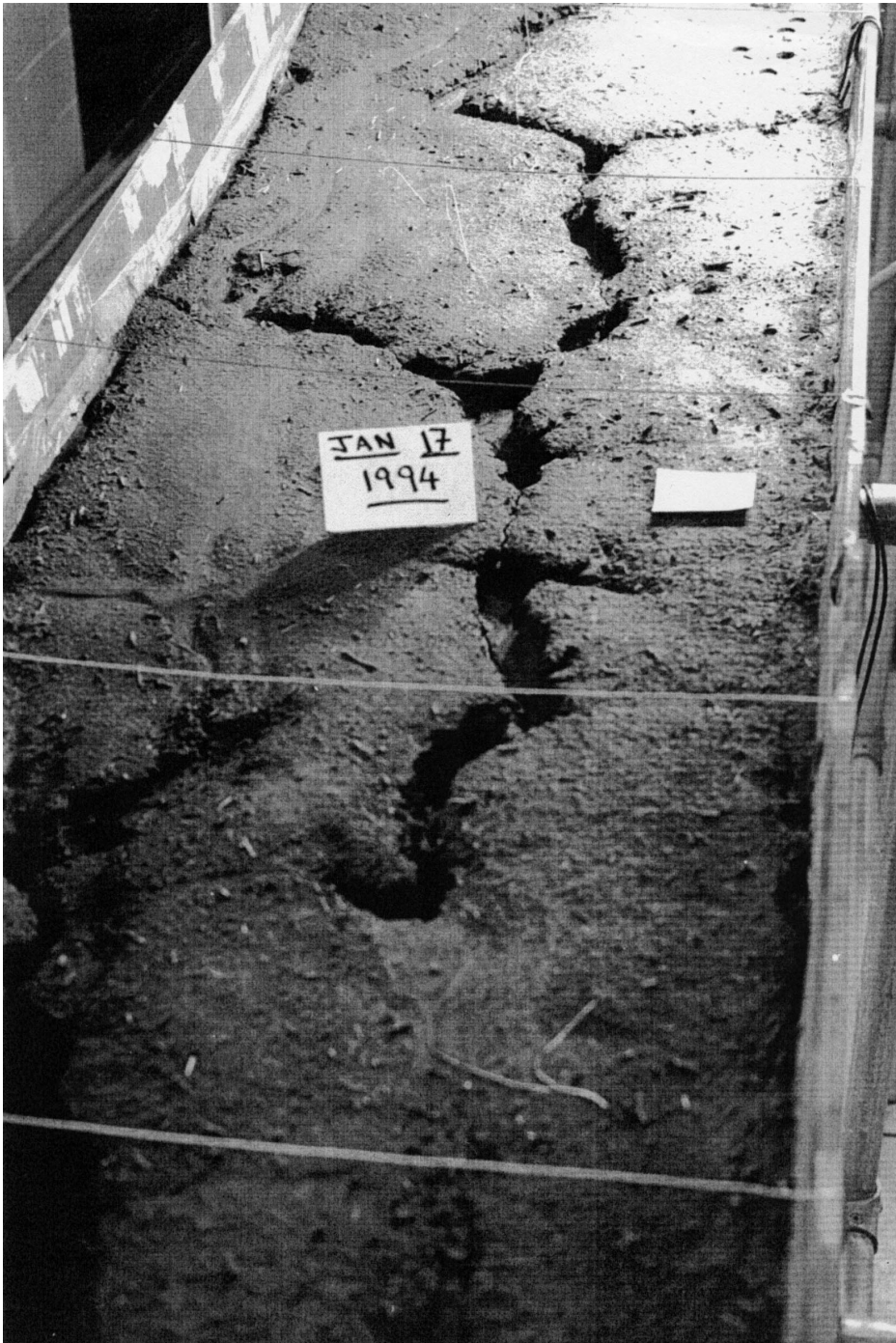
Fig. 6. Micropipes and rills formed in laboratory experiments on Swinton silt loam. Micropipes developed along interstorm desiccation cracks.
