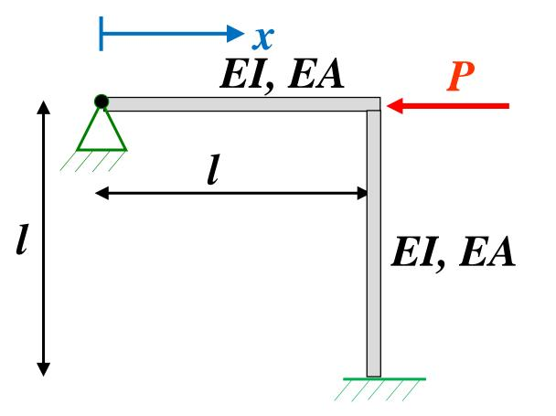
Two identical clamed beam are pinned to a rigid bar as depicted in the figure. Assemble a finite element model to compute the buckling mode of the structure.
