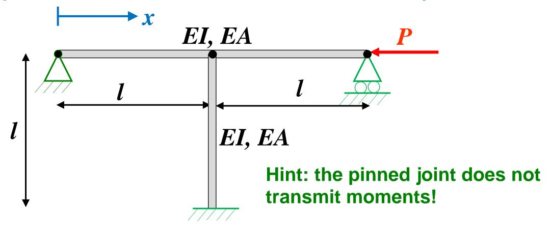
Consider the frame depicted in the figure. The geometry, material properties, and boundary conditions are indicated in the figure. The identical beams are rigidly connected. Assemble a finite element model for computing the buckling load.
