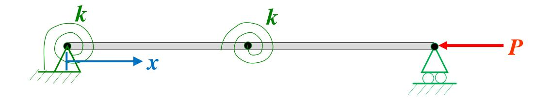
Consider the simply supported beam of length 2l with the geometry and properties depicted in the figure. The beam is under a compressive load. The beam is pinned with another beam of length l at the its center. The other end of this beam is clamped. Assemble a finite element model for the system.
