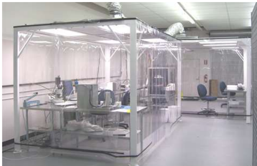
Class 10.000 clean room
