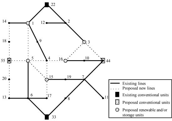
Fig. 3 - Distribution System for the case study
