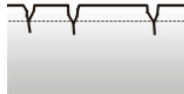
B. SCC Cracks are highly branched
