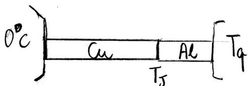
$$\frac{dQ}{dt} = \kappa_{\text{Cu}} \frac{A}{L_{\text{Cu}}} (T_j - 0) \Rightarrow T_j = \frac{L_{\text{Cu}}}{\kappa_{\text{Cu}} A} \frac{dQ}{dt} = \frac{10 \times 10^{-2} \text{ m}}{200 \text{ W} \times 1,00 \times 10^{-4} \text{ m}^2} \frac{83,25 \text{ W}}{\text{m K}} = 416,25 \text{ K}$$
