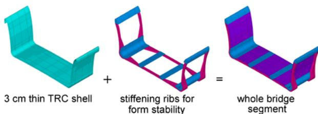
**Figure 3:** Schematic structure of the segments [graphic: Harald Michler, TU Dresden], after [27]
