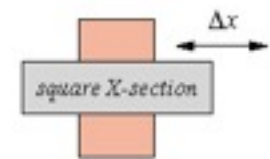
Prismatic (P) joint—1 DOF
