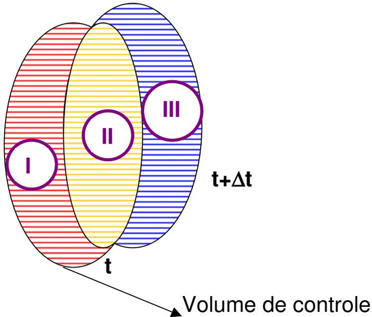
$$\left( \frac{dN}{dT} \right)_{Sist.} = \lim_{\Delta t \rightarrow 0} \left[ \frac{\left( \int_{\forall III} \eta \rho d\forall + \int_{\forall II} \eta \rho d\forall \right)_{t+\Delta t} - \left( \int_{\forall I} \eta \rho d\forall + \int_{\forall II} \eta \rho d\forall \right)_t}{\Delta t} \right]$$
