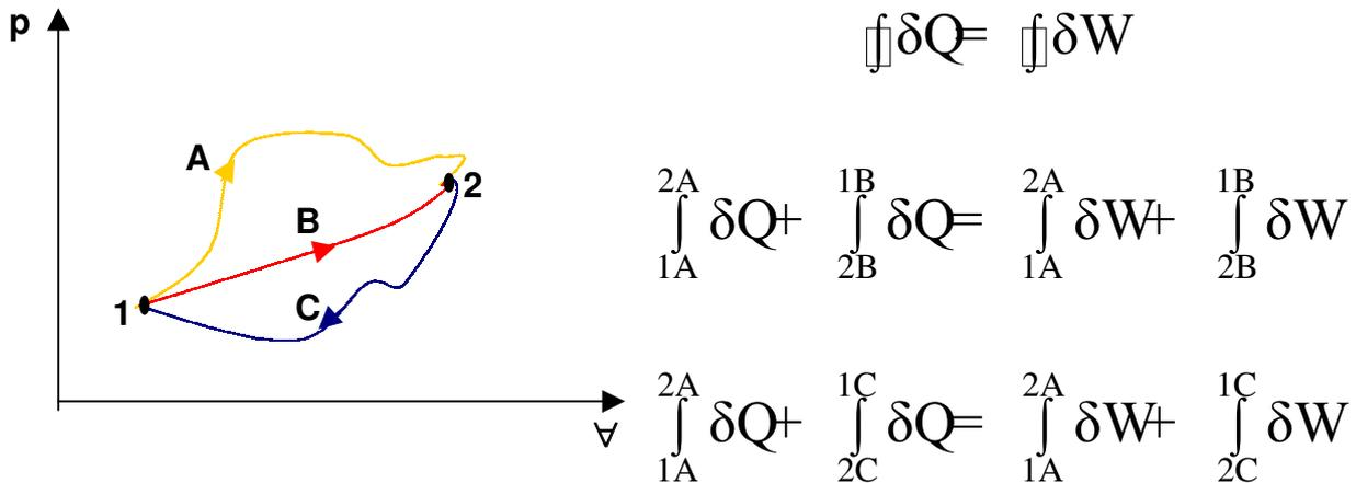
$$\int_{2B}^{1B} \delta Q - \int_{2C}^{1C} \delta Q = \int_{2B}^{1B} \delta W - \int_{2C}^{1C} \delta W \quad \longrightarrow \quad \int_{2B}^{1B} (\delta Q - \delta W) =$$
