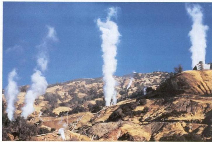
FIGURE 17.2 Geysers Geothermal Field located north of San Francisco, California. The Geysers is the largest geothermal power operation in the world and produces the energy directly from steam.
