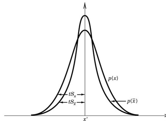
**Figure 4.6** Relationships between  $S_x$  and a distribution of  $x$  and between  $S_{\bar{x}}$  and the true value  $x'$ .
