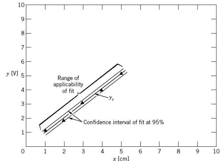
**Figure 4.10** Results of the regression analysis of Example 4.9.
