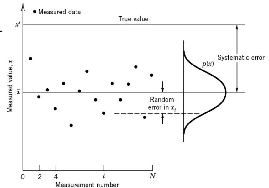
Figure 5.1. Distribution of errors upon repeated measurements.
