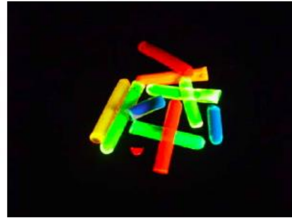
CdSe/ZnS core-shell nanocrystals in a polymer matrix
