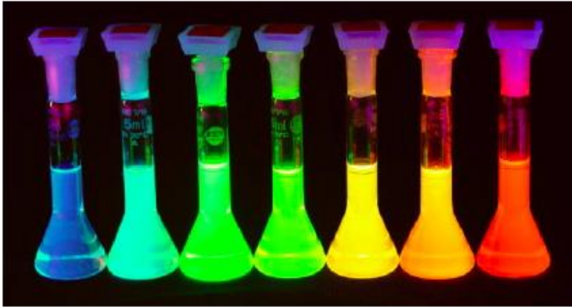
Colloidal solutions of CdSe/ZnS core-shell nanocrystals.
