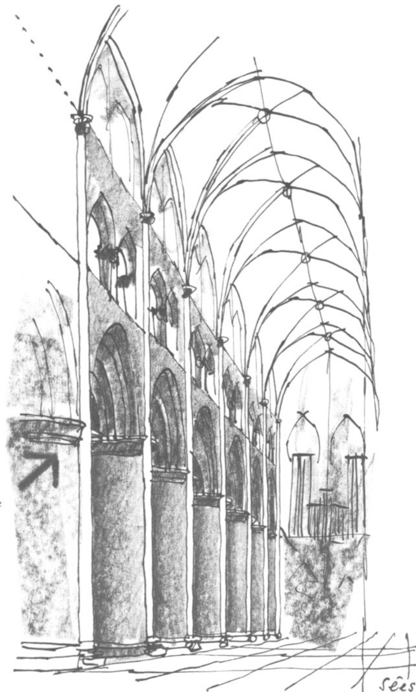
The critical point where the big column lets the slender column pass
