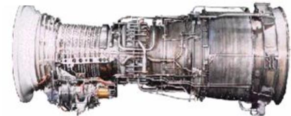
The LM2500 has four major components: a 16-stage, 18:1 pressure ratio compressor with seven stages of variable stators and inlet guide vanes; a fully annular combustor with externally mounted fuel nozzles; a two-stage, air-cooled high-pressure turbine which drives the compressor and the accessory-drive gearbox; and a six-stage, aerodynamically coupled, low-pressure power turbine which is driven by the gas generator's high-energy exhaust gas flow.
