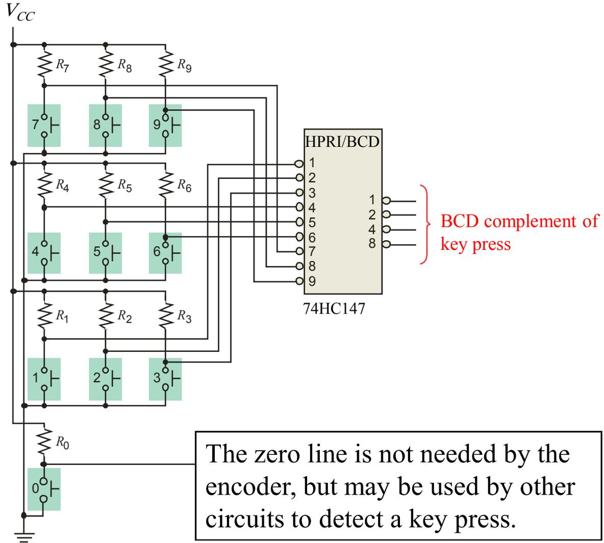
The zero line is not needed by the encoder, but may be used by other circuits to detect a key press.
