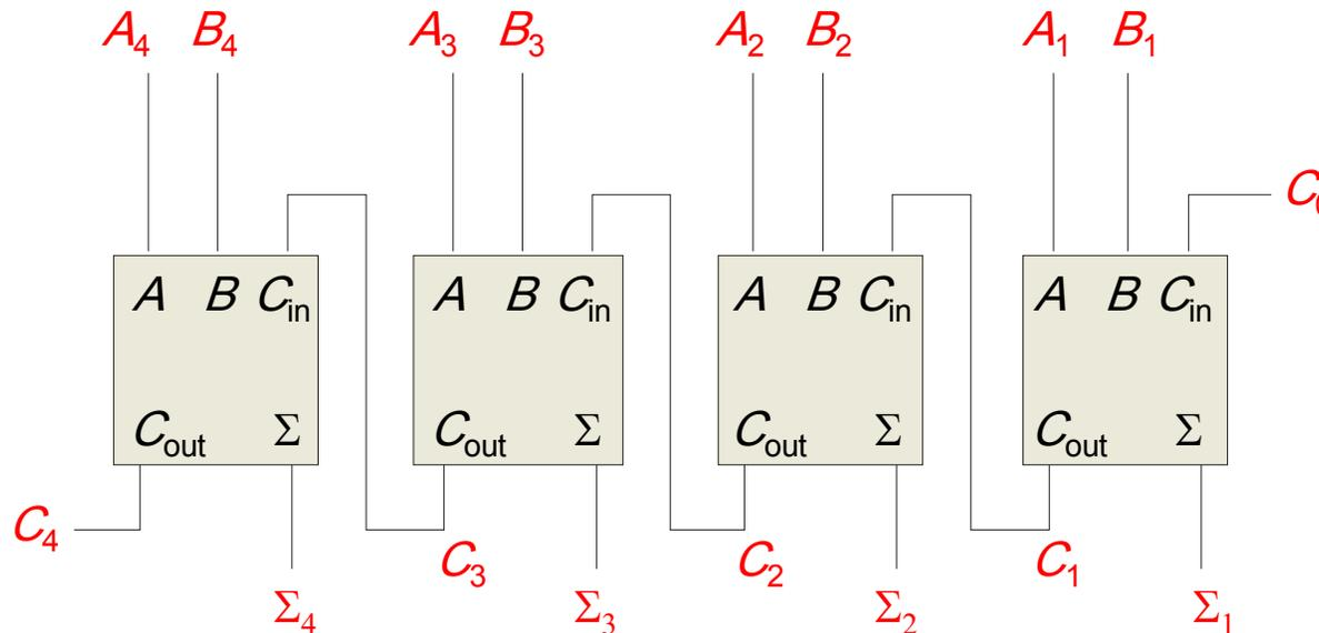
The output carry ( $C_4$ ) is not ready until it propagates through all of the full adders. This is called *ripple carry*, delaying the addition process.
