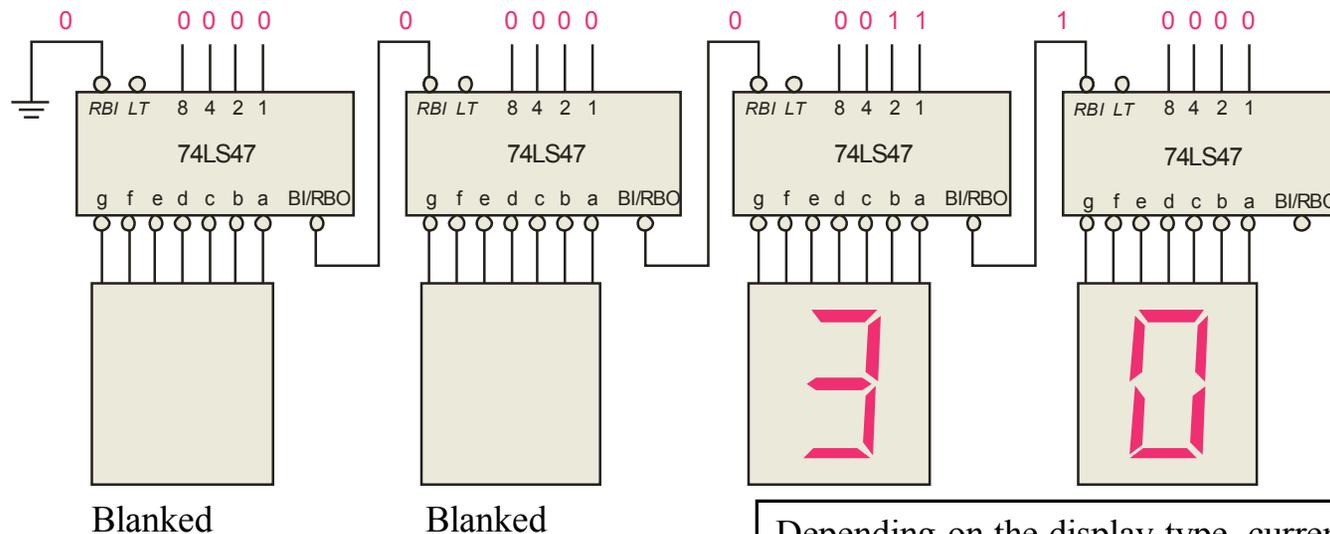
Depending on the display type, current limiting resistors may be required.
