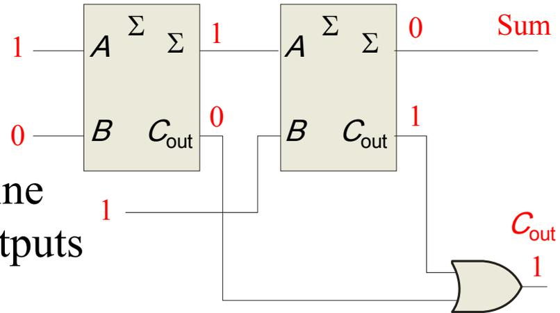
**Solution** The first half-adder has inputs of 1 and 0; therefore the Sum = 1 and the Carry out = 0.
