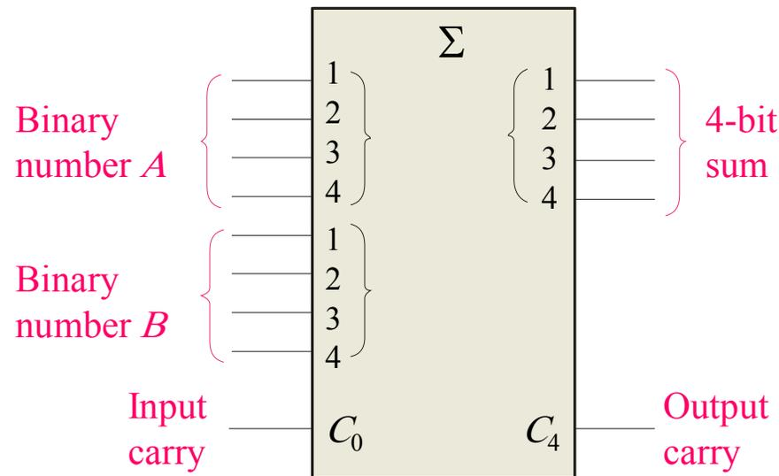
The 74LS283 is an example. It features *look-ahead carry*, which adds logic to minimize the output carry delay. For the 74LS283, the maximum delay to the output carry is 17 ns.
