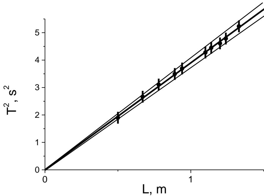
$$T^2 = 4\pi^2(L/g); \quad g_{\text{medio}} = 4\pi^2 \text{ctg} \vartheta_{\text{medio}}; \quad g_{\text{medio}} = 10,12 \text{ m/s}^2;$$
