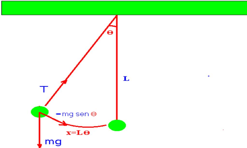
**Pêndulo simples**     $m (d^2x/dt^2) = - mg \text{ sen}\Theta$  ;  $x=L\Theta$ ;
