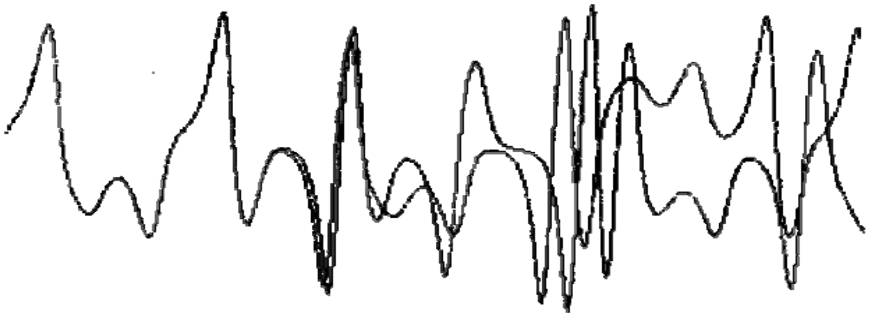
Figure 1: Lorenz's experiment: the difference between the start of these curves is only .000127. (Ian Stewart, Does God Play Dice? The Mathematics of Chaos, pg 141)
