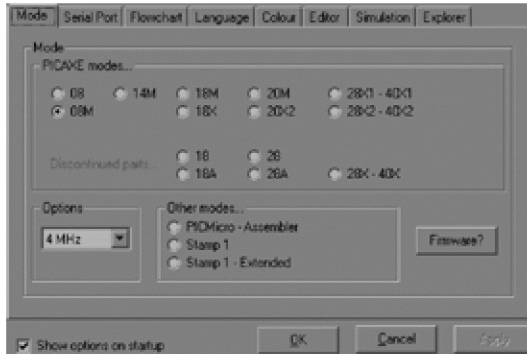
Figure 5-127. This screenshot shows the options window of the PICAXE Program Editor, which you must use to select the type of chip that you intend to program (in our case, the 08M).
