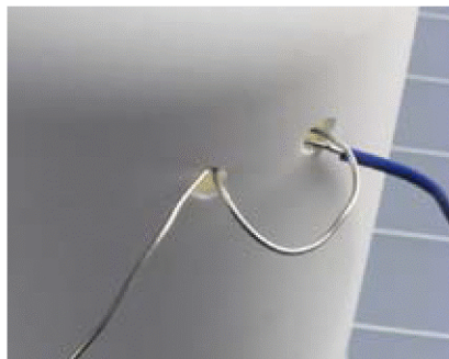
Figure 5-63. The stripped end of the wire is secured through the holes drilled in the bottle.
