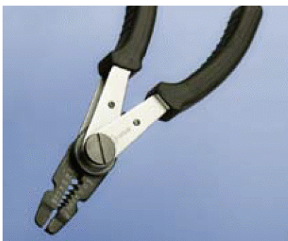
Figure 2-4. To use these wire strippers, insert a piece of insulated wire in the appropriate-sized hole between the jaws, grip the handles, and pull a section of insulation away. See page 45.
