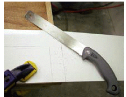
Figure 5-79. This Japanese-style saw cuts when you pull it, rather than when you push it. After some practice, you can use it to make very accurate cuts. Because ABS is so soft, minimal muscle-power is required.
