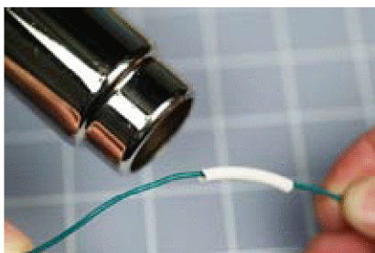
Figure 3-49. Apply heat to the tubing.
