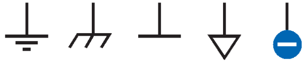
Figure 2-40. All of these symbols are used to mean the same thing: connect the wire to "ground" or "chassis" or the negative side of the power source. The far-right symbol is used in this book.
