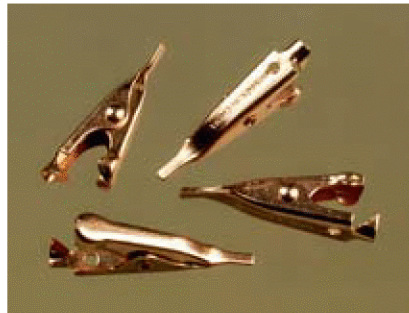
Figure 3-22. These small clips absorb heat to protect components when you're soldering them.
