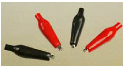
Figure 1-11. Alligator clips inside vinyl sheaths, which reduce the chance of accidental short circuits.
