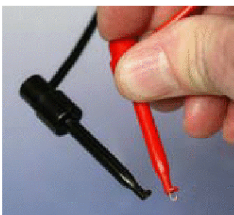
Figure 3-6. These “minigrabber” add-ons for meter leads make it much easier to measure voltage or current. Push the spring-loaded button, and a little copper hook slides out. Attach it to a wire, release the button, and you have your hands free for other tasks. It’s a mystery that meters are not supplied with these grabbers as standard equipment.
