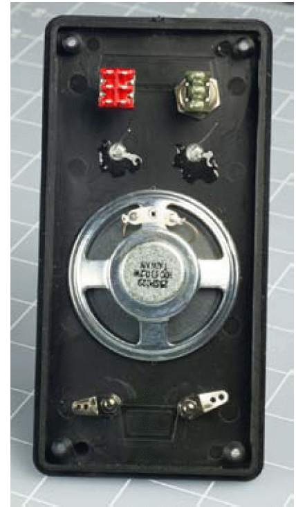
Figure 3-109. Components have been added to the control panel of the project box (seen from the underside). The loudspeaker has been glued in place. Spare glue was dabbed onto the LEDs, just in case. The SPDT on/off switch is at the top right, the DPDT pushbutton is at top left, and the binding posts, which will connect with the network of magnetic sensor switches, are at the bottom.
