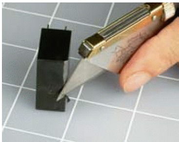
Figure 2-52. To look inside a sealed relay, shave the top edges of the plastic package with a utility knife til you open a thin crack.
