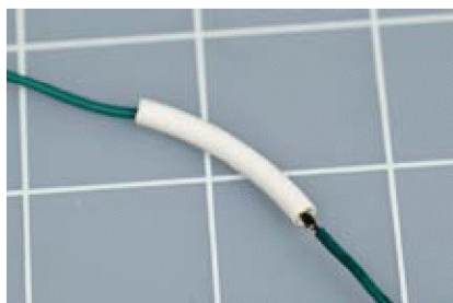
Figure 3-48. Slip the tubing over your wire joint.
