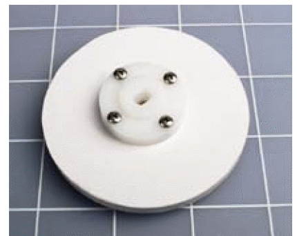
Figure 5-93. A 3-inch wheel is screwed to the disc that mates with the drive shaft of the motor.
