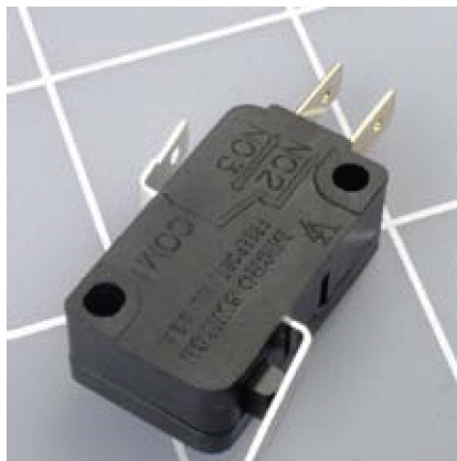
Figure 5-74. A microswitch has a small button (at the front, righthand side in this picture) that is often actuated by a pivoted metal lever. The switch can respond to a very light pressure, but can handle relatively high currents.
