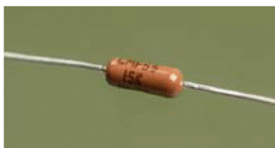
Figure 1-41. Some modern resistors have their values printed on them, although you may need a magnifier to read them. This 15K resistor is less than half an inch long.
