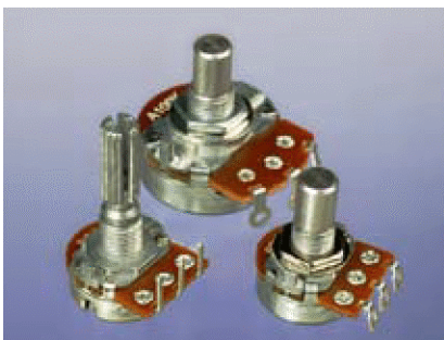
Figure 1-13. Potentiometers come in many shapes and sizes, with different lengths of shafts intended for different types of knobs. For our purposes, any style will do, but the larger-sized ones are easier to play with.
