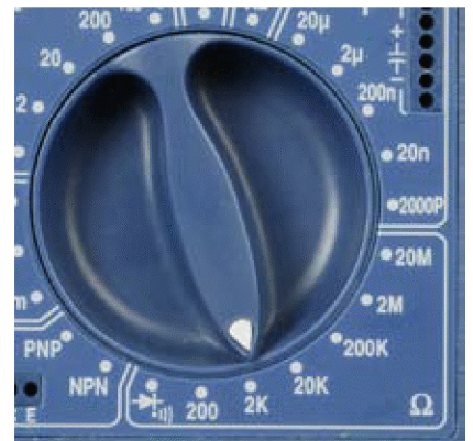
Figure 1-25. To measure ohms, turn the dial to the ohm (omega) symbol. On an autoranging meter, you can then press the Range button repeatedly to display different ranges of resistance, or simply touch the probes to a resistance and wait for the meter to choose a range automatically. A manual meter requires you to select the range with the dial (you should set it to 100K or higher, to measure skin resistance). If you don't get a meaningful reading, try a different range.
