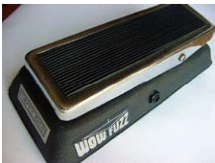
Figure 5-53. This Vox Wow-Fuzz pedal was one of the early stomp boxes, which deliberately induced the kind of distortion that audio engineers had been trying to get rid of for decades.
