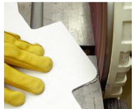
Figure 5-82. A belt sander or disc sander is the ideal tool for rounding corners when working with ABS plastic.
