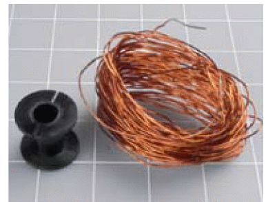
Figure 5-47. The audio crossover coil consists of a plastic spool and some wire. Nothing more.
