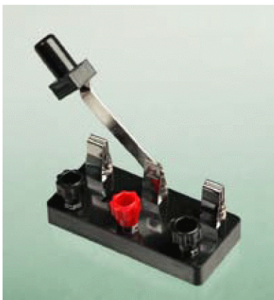
Figure 2-24. This primitive-looking single-pole, double-throw switch does exactly the same thing as the toggle switches in Figures 2-23 and 2-27.
