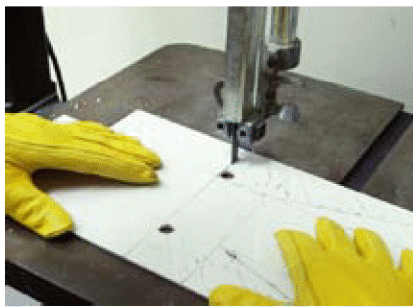
Figure 5-77. A band saw is an ideal tool for cutting complex shapes out of ABS plastic. You can often find them secondhand for under $200.
