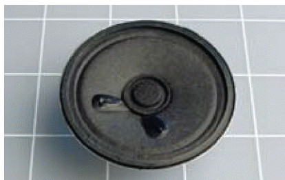
Figure 5-25. Loudspeaker ready for creative destruction.
