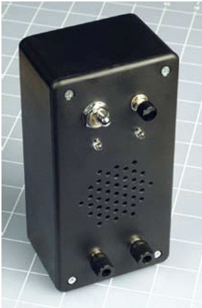
Figure 3-114. The intrusion alarm completed and in its project box.
