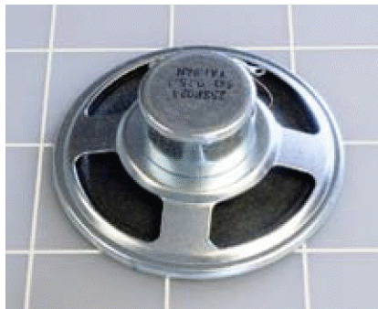
Figure 5-24. A 2-inch loudspeaker can be instructively destroyed with a utility knife or X-Acto blade.
