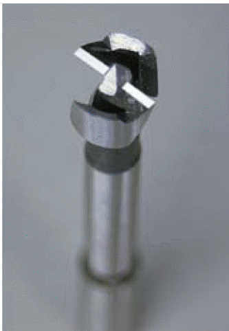
Figure 5-83. A Forstner drill bit makes clean, precise holes; a large regular drill bit will chew up ABS plastic and make a mess.
