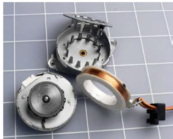
Figure 5-115. When a stepper motor is broken open, this is what you're likely to find. On the left, the rotor of the motor, which has a magnetized band around its circumference, is still attached to the lower half of the casing. On the right, the upper half of the casing has been opened, and the coil has been removed (actually the winding you can see consists of two coils, wound in opposite directions). The spikes are the magnetic cores that exert force on the rotor.
