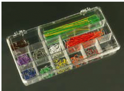
Figure 2-9. Precut wires with stripped ends can save a lot of time and trouble—if you don't mind paying a little extra.
