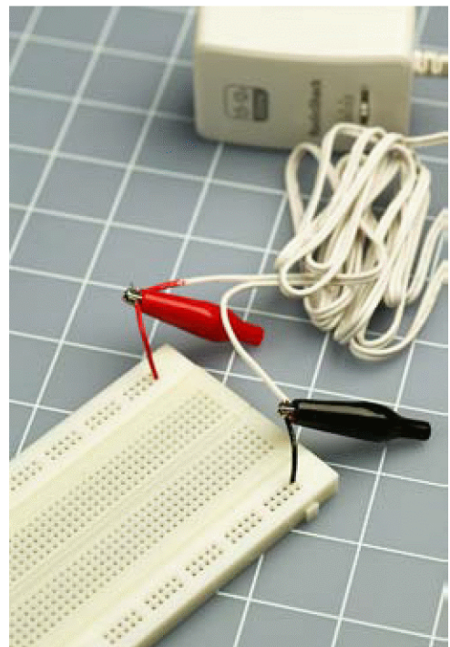
Figure 2-75. If your breadboard doesn't have screw terminals, insert two short pieces of solid-core wire with stripped ends and then attach the stranded wires from the adapter using alligator clips.
