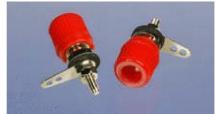
Figure 3-27. These terminals, also known as binding posts, enable a solderless connection with wires that have stripped ends. Also available in black.
