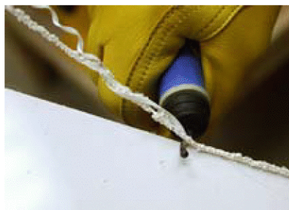
Figure 5-81. A deburring tool will clean and bevel the sawn edge of a piece of plastic in just a couple of quick strokes.
