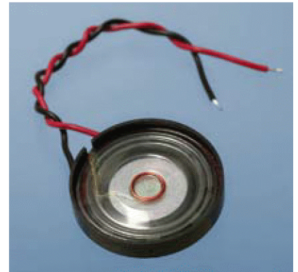
Figure 2-16. This miniature loudspeaker, just over 1 inch in diameter, is useful for verifying audio output direct from transistor circuits.
