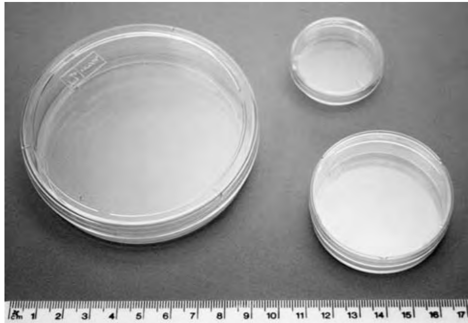
Fig. 8.3. Petri Dishes. Illustrated are dishes of 3.5-cm, 5-cm, and 9-cm diameter. Square Petri dishes are also available, with dimensions 9 \times 9 cm. A grid pattern can be provided to help in scanning the dish—for example, in counting colonies—but can interfere with automatic colony counting.
