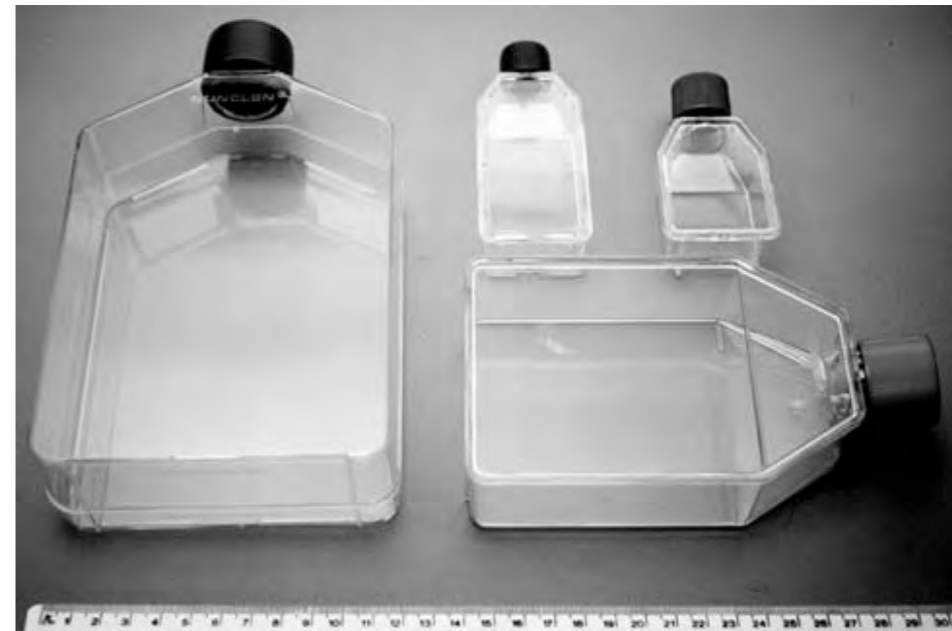
Fig. 8.4. Plastic Flasks. Sizes illustrated are 10 and 25 cm 2 (Falcon, B-D Biosciences), 75 cm 2 (Corning), and 185 cm 2 (Nalge Nunc) (see Table 8.1 for representative sizes and capacities).
