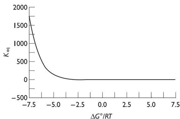
**Fig. 4.10** Variation of  $K_{\text{eq}}$  with  $\Delta G^\circ$ . Note that  $K_{\text{eq}}$  is a function of the negative logarithm of  $\Delta G^\circ$ . When  $\Delta G^\circ$  is large and negative,  $K_{\text{eq}}$  is very large. When  $\Delta G^\circ$  is large and positive,  $K_{\text{eq}}$  is very small. In most biochemical reactions  $\Delta G^\circ$  will fall within the range shown here.
