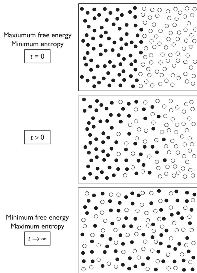
**Fig. 4.4** Mixing. At time  $t = 0$ , when the partition is removed, the liquids are completely separate. The liquids are miscible so mixing occurs. After a sufficiently long time, the liquids are completely mixed. The unmixed state has a maximum of free energy for the system and a minimum of entropy. The completely mixed state has a minimum of free energy and a maximum of entropy. Based on Fig. 1.5 of van Holde (1985).
