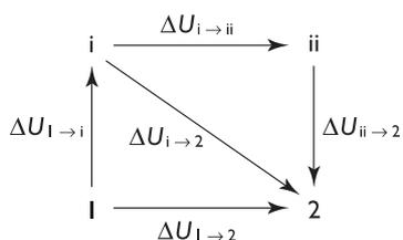
**Fig. 2.3** Thermodynamic cycle.
