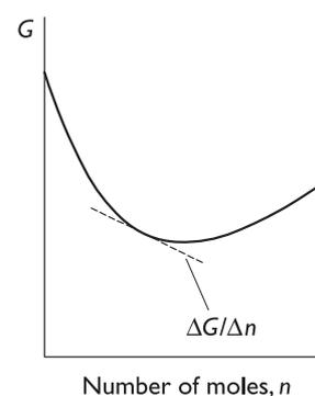
**Fig. 4.8** Thermodynamic potential and solute concentration. The Gibbs free energy of a solute varies with concentration. The chemical potential measures the rate of change of  $G$  with  $n$ , or the slope of the curve at a given value of  $n$  ( $\Delta G/\Delta n$ ). Note that  $G$  can decrease or increase on increases in concentration.
