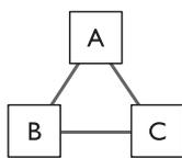
**Fig. 2.1** The Zeroth Law of Thermodynamics. If three systems, A, B and C, are in physical contact, at equilibrium all three will have the same temperature. The concept of equilibrium is discussed in depth in Chapter 4.
