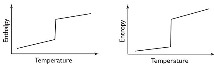
**Fig. 4.5** First-order phase transition. The graphs show the behavior of the enthalpy and entropy functions versus temperature. Both of these thermodynamic quantities are *discontinuous* at the transition temperature, as is  $C_p$ .
