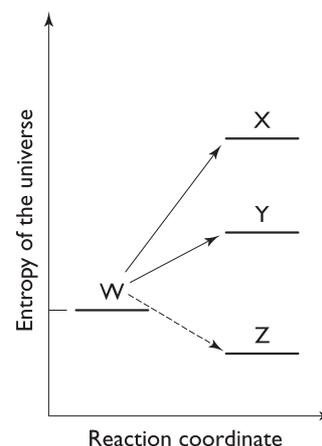
**Fig. 3.4** The Second Law of Thermodynamics. No process will occur spontaneously unless it is accompanied by an increase in the entropy of the universe. This applies to an isolated system, a closed system, and an open system.
