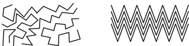
**Fig. 3.3** Schematic diagram of a rubber band in the unstretched (equilibrium) state (left) and stretched state (right). In the unstretched state, the molecules are highly disordered. When the band is stretched, the molecules form a relatively orderly array. The entropy of the molecules is lower in the stretched state than in the unstretched state.
