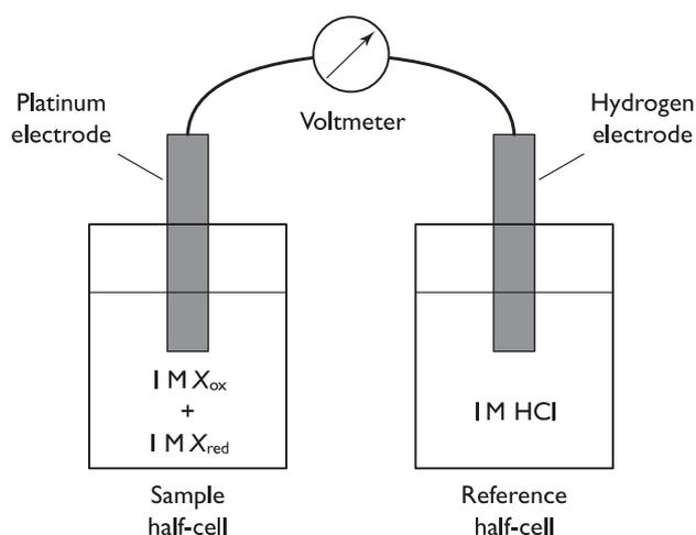
**Fig. 4.14** Measurement of the standard redox potential. This device can be used to measure the standard redox potential of a compound. The hydrogen electrode in the reference cell contains 1 atm  $\text{H}_2(\text{g})$ .
