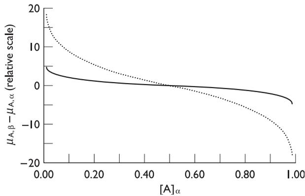
**Fig. 4.9** Chemical potential difference as a function of concentration. The figure illustrates the behavior of the left-hand side of Eqn. (4.7) when the total concentration of A is fixed;  $[A]_\alpha + [A]_\beta = \text{constant}$ . The dashed line represents a change in temperature.
