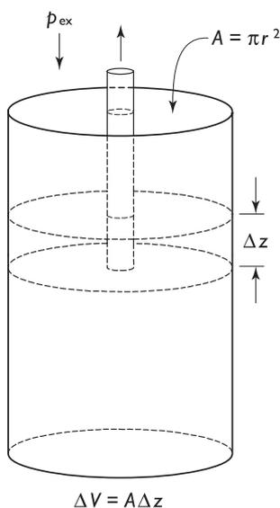
**Fig. 2.6** Gas-filled cylinder. There is a constant external pressure,  $p_{\text{ex}}$ . For a change in position of the piston,  $\Delta z$ , there is a corresponding change in volume,  $\Delta V$ . The work done *by* the system is  $w = -p_{\text{ex}}\Delta V$ . If  $\Delta V$  is negative, if the gas in the cylinder is compressed, there is a positive contribution to  $\Delta U$ .
