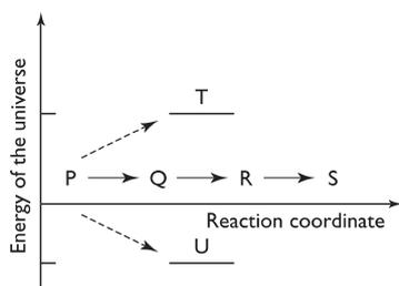
**Fig. 2.2** The First Law of Thermodynamics. The total energy of the universe is constant, no matter what changes occur within. This principle also applies to an isolated system. Moreover, it is no less applicable to an open system or a closed system, as long as a complete account can be made of energy exchanged with the surroundings.
