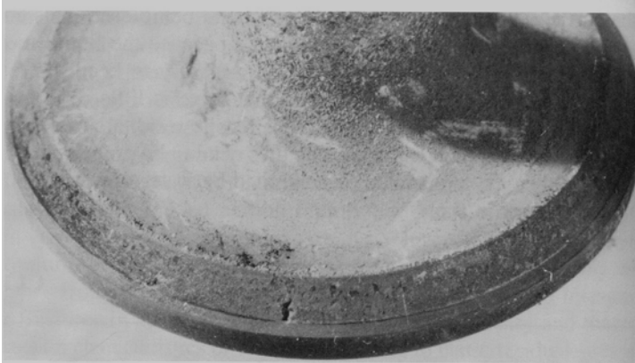
Fig. 11(a). Incipient burning on the valve face of an automotive engine exhaust valve caused by microporosity in the hard facing alloy. Macrograph at about 2\frac{1}{2}\times .
