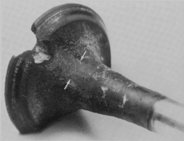
Fig. 11(a). Incipient burning on the valve face of an automotive engine exhaust valve caused by microporosity in the hard facing alloy. Macrograph at about 2\frac{1}{2}\times .
