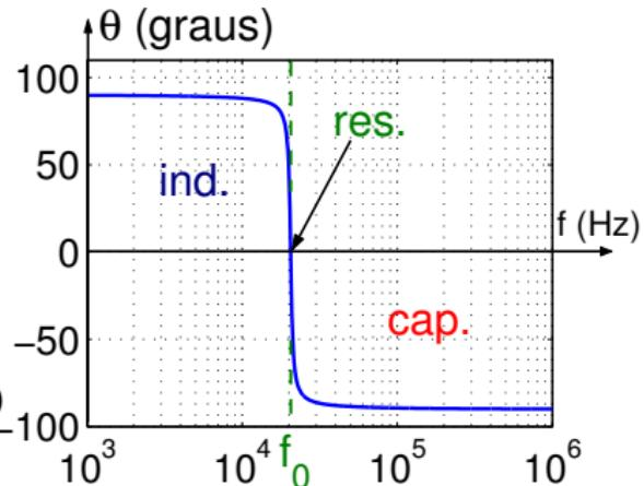
$$\text{Freq. de ressonância: } f_r = f_0 = \frac{1}{2\pi\sqrt{LC}} \approx 20,55 \text{ kHz}$$
