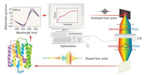
**In the loop.** A feedback loop is used to control isomerization of bacteriorhodopsin. An initial laser control field is created with a pulse shaper (on the right) and is then applied to the protein sample. The action of the control pulse, measured as the difference spectrum of the sample, is used by a learning algorithm to produce an improved field. Repeated excursions around the loop result in an optimum control.
