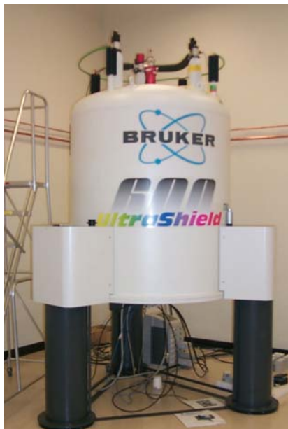
Figure 11 - 9, Bruker 600 MHz 89 mm wide bore ultra shield magnet.
