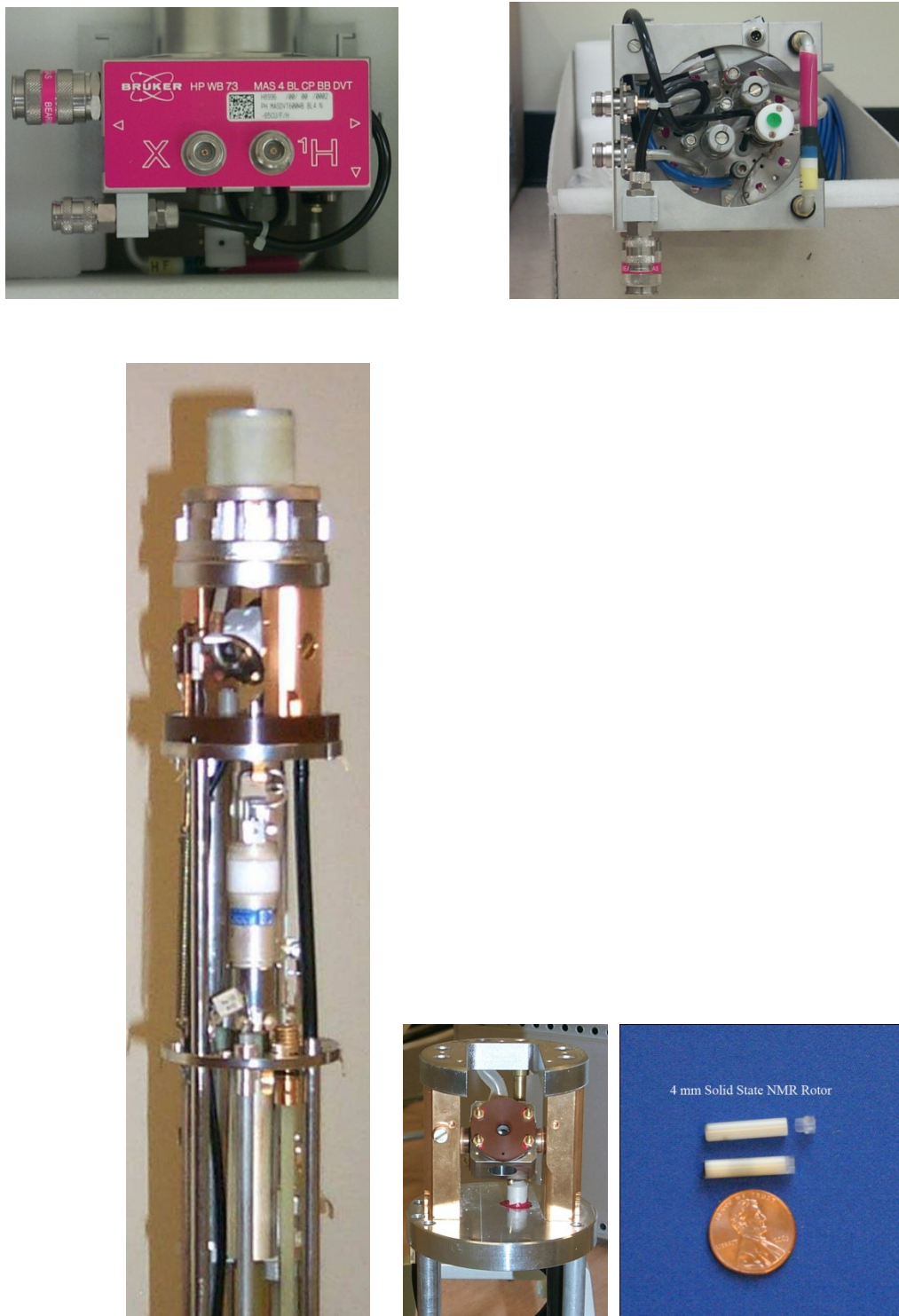
Figure 4 – 11. From top left: Bruker 4 mm HFX solid state NMR probe base, bottom of the probe; probe head for wide bore magnet; Spinning test station; 4 mm solid state NMR sample rotor.
