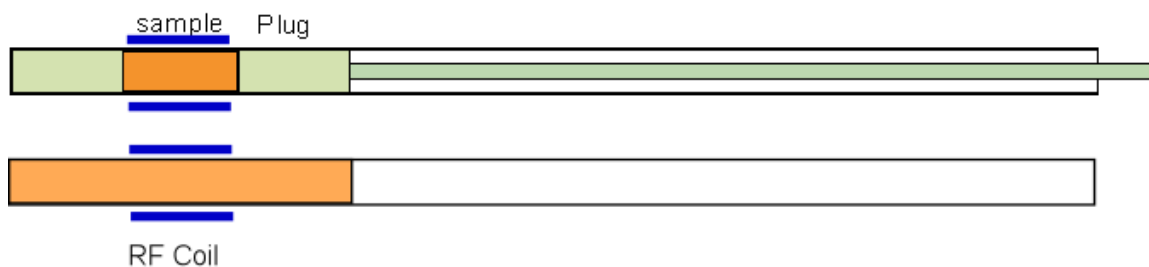
Figure 6 – 1. From the top: Shigemi NMR tube, the magnetic susceptibility of the glass is matched to that of the solvent. A regular NMR tube needs three times of volume. It allows us to use a smaller sample volume, save solvent, more concentrated sample within the RF coil.
