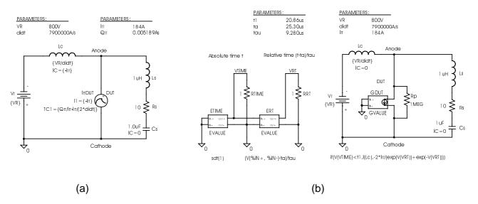
*Fig. 5: Pspice circuits for calculating reverse overvoltage, using the exponential (a) and the sech (b) models*
