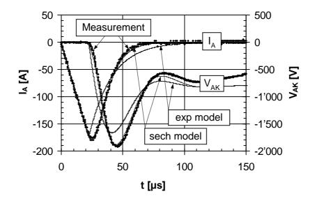
Fig. 6: Turn-off transients for a 5STP 18L4200 thyristor at 125 °C and -7.9 A/ $\mu$ s with a snubber of 10  $\Omega$ /1.0  $\mu$ F and a reverse voltage of about -800 V. The measured waveform is compared with model transients adjusted for equal di/dt, Q<sub>rr</sub> and I<sub>rr</sub>.
