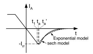
*Fig. 4:* Comparison of exponential and sech models, adjusted to exhibit the same di/dt,  $Q_{rr}$  and  $I_{rr}$
