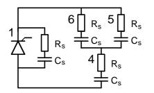
Fig. 10: Simplified equivalent circuit during turn-off of Thyristor 1
