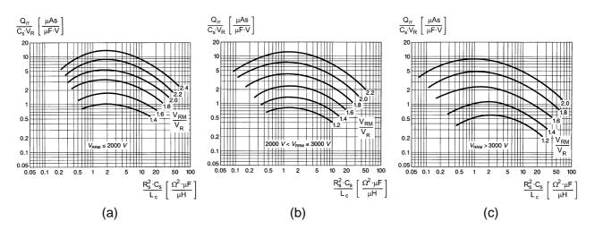
Fig. 7: Curves for determining the optimum RC snubber values of ABB phase control thyristors. The curves are valid for thyristors with  $V_{RRM}$  ratings below 2000 V (a), between 2000 and 3000 V (b) and above 3000 V (c). For diodes, similar curves apply but they depend somewhat more on the specifics of the design of the individual part number.
