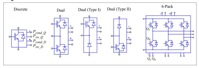
In the images, beside the IGBT and diode terminal nodes, there are four extra nodes from the top to the bottom (or from the left to the right on the top for the 6-pack package). They are the nodes for transistor conductor losses  $P_{cond\_Q}$  (the node with a circle), for transistor switching losses  $P_{sw\_Q}$ , for diode conductor losses  $P_{cond\_D}$  (the node with a square), and for diode switching losses  $P_{sw\_D}$ , respectively.
