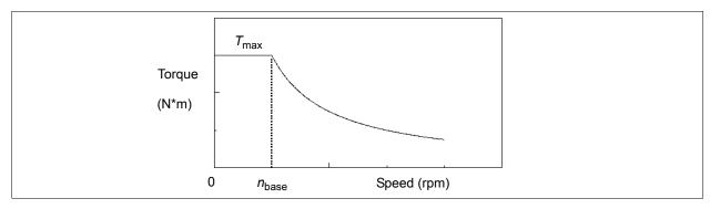
When the mechanical speed is less than the base speed  $n_{\text{base}}$ , the load torque is:
