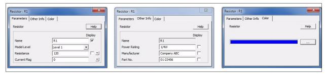
The parameters in the **Parameters** tab are used in the simulation. The information in the **Other Info** tab, on the other hand, is not used in the simulation. It is for reporting purposes only and will appear in the parts list in **View** >> **Element List** in PSIM. Information such as device rating, manufacturer, and part number can be stored under the **Other Info** tab.
