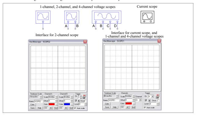
The 1-channel and 4-channel voltage scope and the current scope have the same interface. For the 4-channel scope, the channel can be selected through the drop-down channel selection, and the settings apply that the channel selected.
