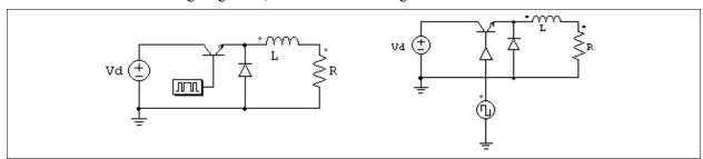
If the switch is controlled by a control circuit signal, as shown in the circuit on the right side, an on-off switch controller must be used at the gate node.
