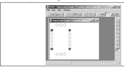
In the window, the diamonds marked red are the connection nodes of the subcircuit block, in exactly the same positions as appearing in the main circuit.
