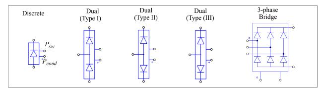
In the images, beside the diode anode and cathode terminals, there are two extra nodes. The node with a dot is for the diode conduction losses  $P_{cond}$ , and the node without a dot is for the diode switching losses  $P_{sw}$ .
