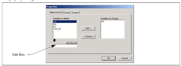
All the data variables available for display are in the *Variables Available* box, and the variables currently being displayed are in the *Variables for Display* box. After a variable is highlighted in the *Variables Available* box, it can be added to the *Variables for Display* box by clicking on "Add ->". Similarly, a variable can be removed from display by highlighting the variable and clicking on "<- Remove".
