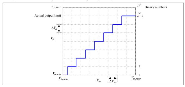
The number of bits determines the quantization resolution. The input range,  $V_{in,max}$  -  $V_{in,min}$ , is divided into  $2^{N}$  stages, with the width of each stage as:
