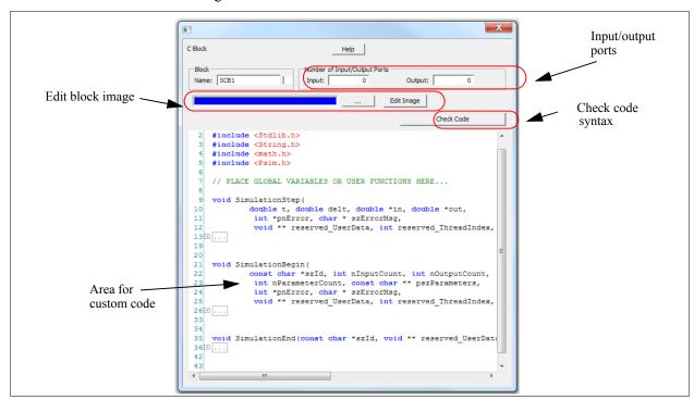
Number of input and output ports of the C block is defined in the *Number of Input/Output Ports* section. If the number of ports is changed, the image of the block in the schematic will change accordingly.
