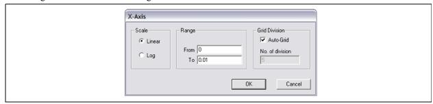
If the *Auto-Grid* box is checked, the number of axis divisions will be automatically determined. The data range and grid division, however, can be manually set.
