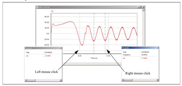
Once **Measure** is selected, an individual curve can be selected by clicking on the pull-down menu on the Measure toolbar. The functions, **Max**, **Min**, **Next Max**, **Next Min**, **Avg**, **and rms**, can be used to evaluate the curve. Note that these functions are only enabled in the **Measure** mode.
