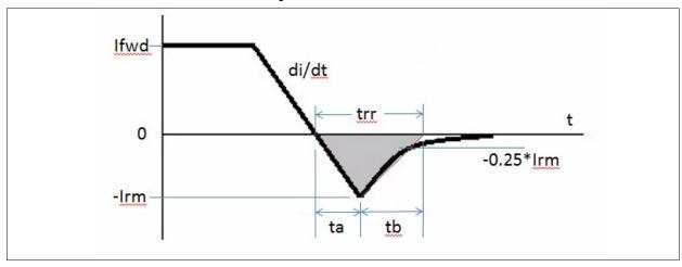
The reverse recovery time *trr* consists of two parts: *ta* and *tb*. During the period *ta*, the current increases from 0 to *-Irm*. Based on JEDEC (Joint Electron Device Engineering Council), *tb* is defined as the interval from the time of *-Irm* to the time when the straight line from *-Irm* through -0.25\**Irm* (in red in the diagram) intersects with the time axis.
