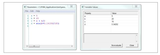
The function **Show Values** provides a very convenient way of checking the calculation.
