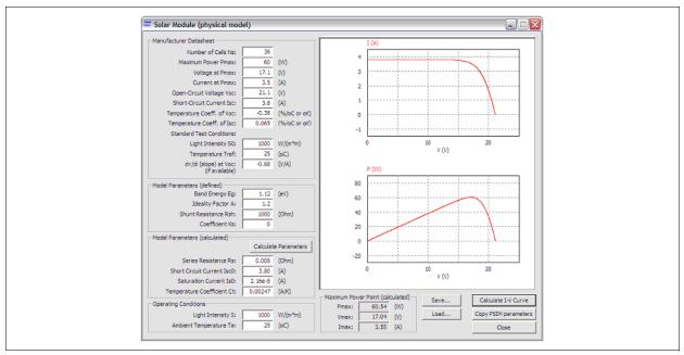
Some of the parameters of the physical model can be obtained from manufacturer datasheet, and the rest of the parameters can be obtained by trial-and-error. A utility tool *Solar Module (physical model)* under the **Utilities**
