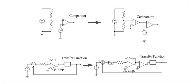
It should be noted that, in PSIM, the power circuit and the control circuit are solved separately. There is one time step delay between the power and the control circuit solutions.
