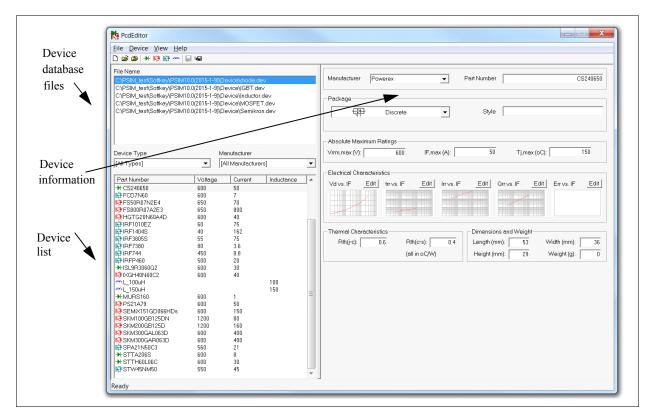
On the left are the device database files that are loaded into the database editor, and the list of the devices. The devices can be displayed based on either **Device Type** or **Manufacturer**. Also, the device list can be sorted by **Part Number**, **Voltage** rating, or **Current** rating, by clicking on the title bars of the list.
