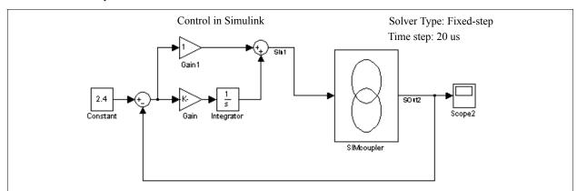
It is recommended that Simulink use the same time step as PSIM, although we have found that, even if the Simulink time step is slightly larger than PSIM time step, satisfactory results are obtained. In this case, for
