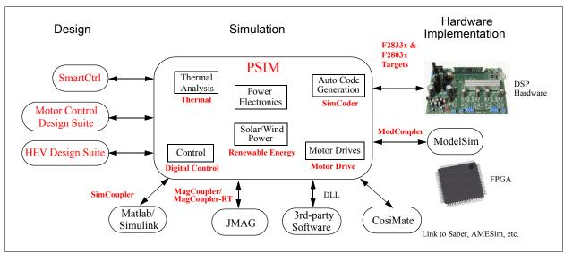
The PSIM simulation environment consists of the circuit schematic program PSIM, the simulator engine, and the waveform processing program SIMVIEW<sup>1</sup>. The simulation process is illustrated as follows.
