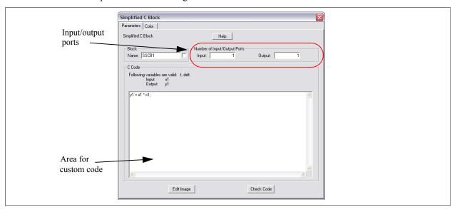
The number of input and output ports of the ports is defined in the *Number of Input/Output Ports* section. After the number of ports is changed, the image of the block in the schematic will change accordingly.
