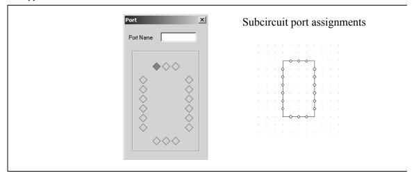
The diamonds on the four sides represent the connection nodes and the positions of the subcircuit. They correspond to the connection nodes of the subcircuit block on the right. There are no diamonds at the four corners since connections to the corners are not permitted.
