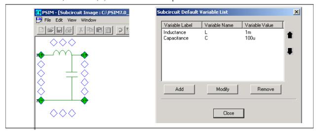
Then from **Subcircuit** >> **Edit Default Variable List**, add the variables L and C as the default variables. This step is necessary as the new element obtains the parameter information from the default variable list. The default variable list window should appears as follows.
