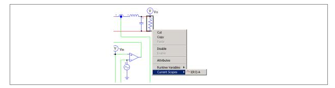
If the element has multiple current flags, under the *Current Scopes* menu, there will be multiply branch currents, one corresponding to each current flag.
