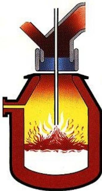
*Figure 3: Schematic drawing of BOS process and the turbulence generated which causes refractory erosion*
