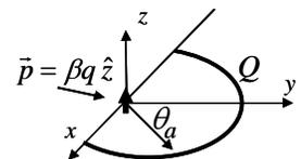
$$E_y = \frac{-1}{4\pi\epsilon_0} \int_{-\pi/2}^{+\pi/2} \frac{\lambda a d\theta}{a^2} \cos\theta \quad \text{onde} \quad \lambda = \frac{Q}{\pi a} \quad E_y = \frac{-1}{4\pi\epsilon_0} \frac{Q}{\pi a^2} \int_{-\pi/2}^{+\pi/2} \cos\theta d\theta = \frac{-1}{2\pi\epsilon_0} \frac{Q}{\pi a^2}$$
