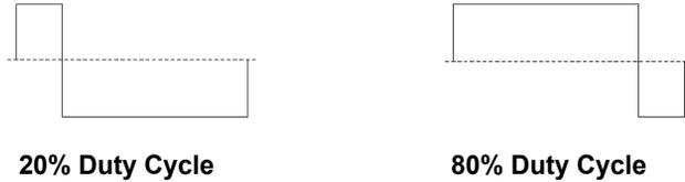
(See Pulse Waveforms, on page 98 for information about duty cycle for pulse waveforms.)
