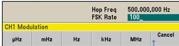
*At this point, the waveform generator outputs an FSK waveform.*
