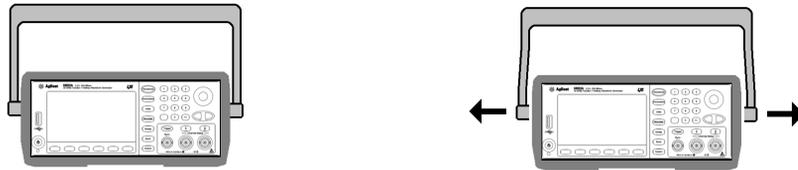
To remove the handle, rotate it to vertical and pull the ends outward.
