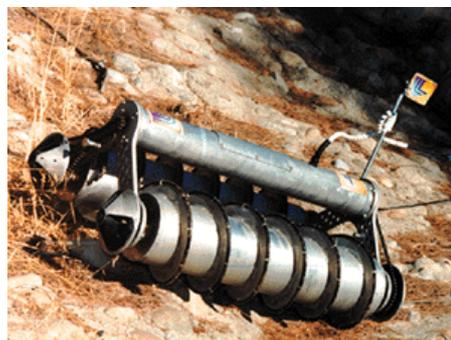
Figura 2.18 Robot “Spiral Track” [21]
