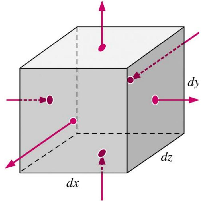
$$(\rho u)_{\text{centro da face direita}} = \rho u + \frac{\partial (\rho u)}{\partial x} \frac{dx}{2} + \frac{1}{2!} \frac{\partial^2 (\rho u)}{\partial x^2} \left( \frac{dx}{2} \right)^2 + \dots$$
