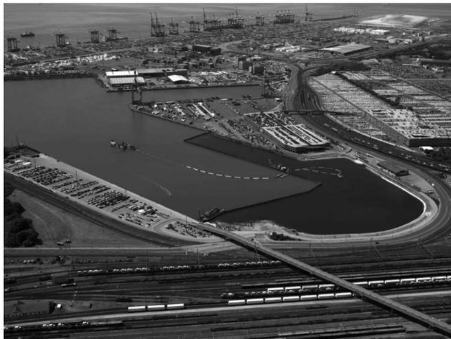
**Fig. 1.** Air photo of the East Harbor construction site, where 180,000 m<sup>3</sup> of harbor mud were relocated behind a sheet pile wall (photo used with permission of bremenports GmbH & Co. KG)
