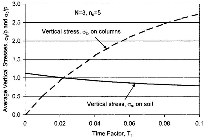
FIG. 3. Vertical Stresses on Soil and Columns with Time
