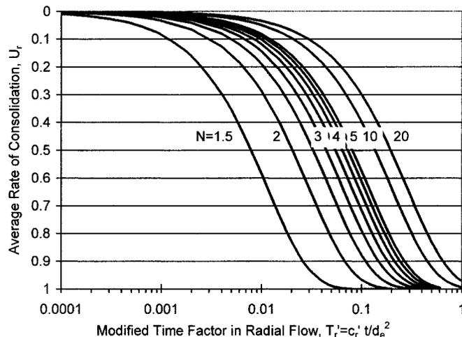
FIG. 8. Rate of Consolidation in Radial Flow
