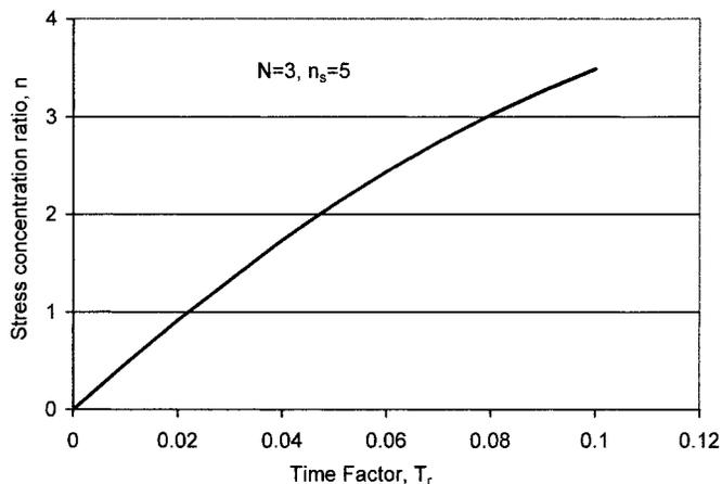
FIG. 4. Stress Concentration Ratio with Time
