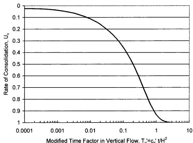
FIG. 7. Rate of Consolidation in Vertical Flow
