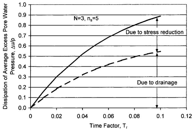
FIG. 5. Dissipation of Excess Pore Water Pressure
