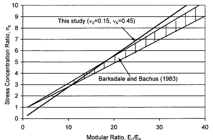
FIG. 2. Relationship between Stress Concentration Ratio and Modular Ratio
