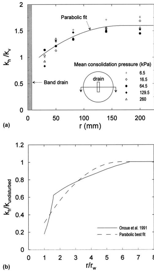
**Fig. 1.** (a) Ratio of horizontal to vertical permeability along radial distance from drain in large scale consolidometer [original data from Indraratna and Redana (1998b)]; (b) proposed horizontal permeability distribution for isotropic soil [original data from Onoue et al. (1991)]
