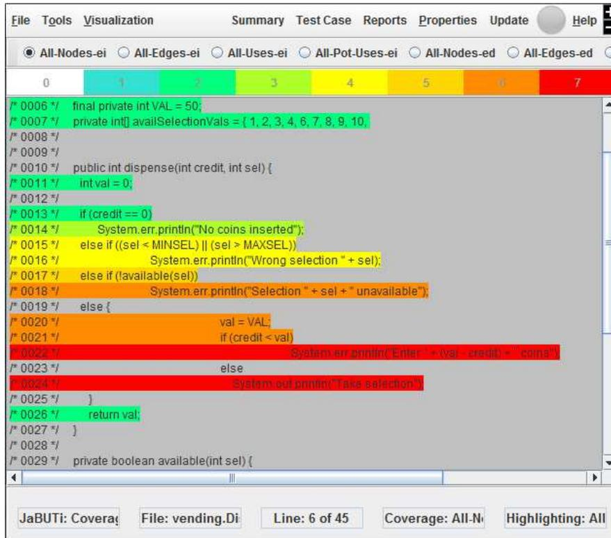
Figure 7: Dispenser.dispense method: source code prioritized w.r.t. All-Pri-Nodes criterion.
