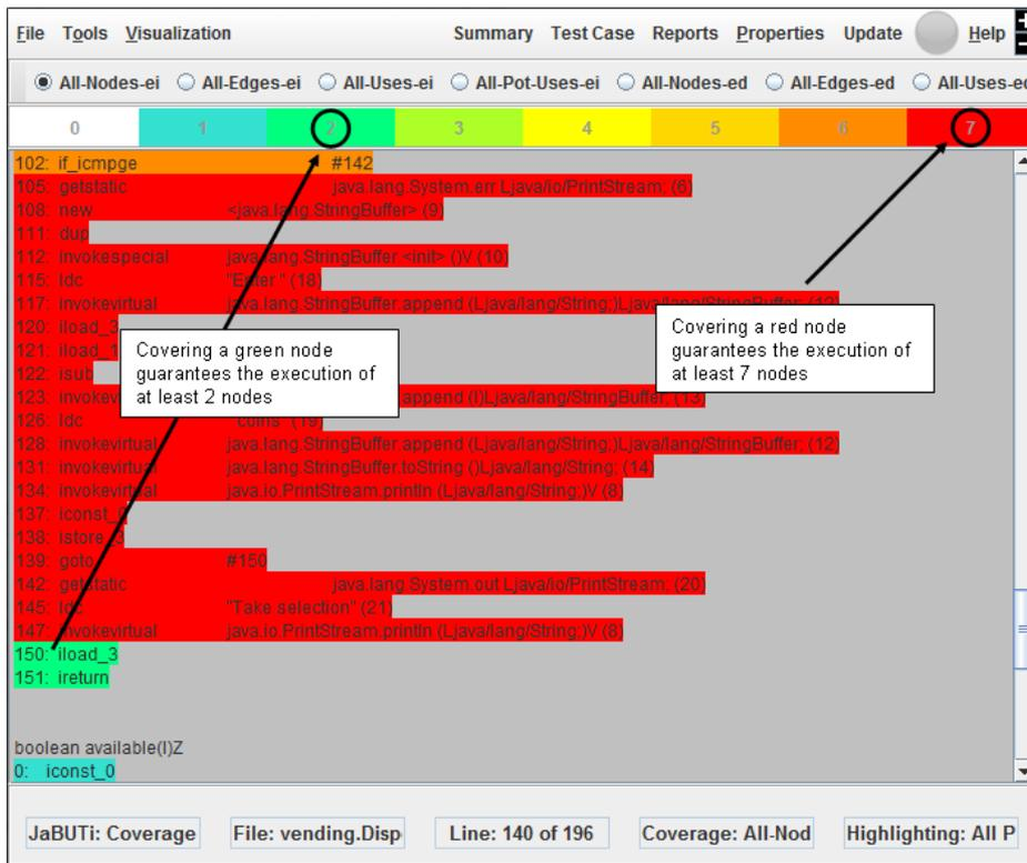
Figure 5: Dispenser.dispenser method: bytecode prioritized w.r.t. All-Pri-Nodes criterion.
