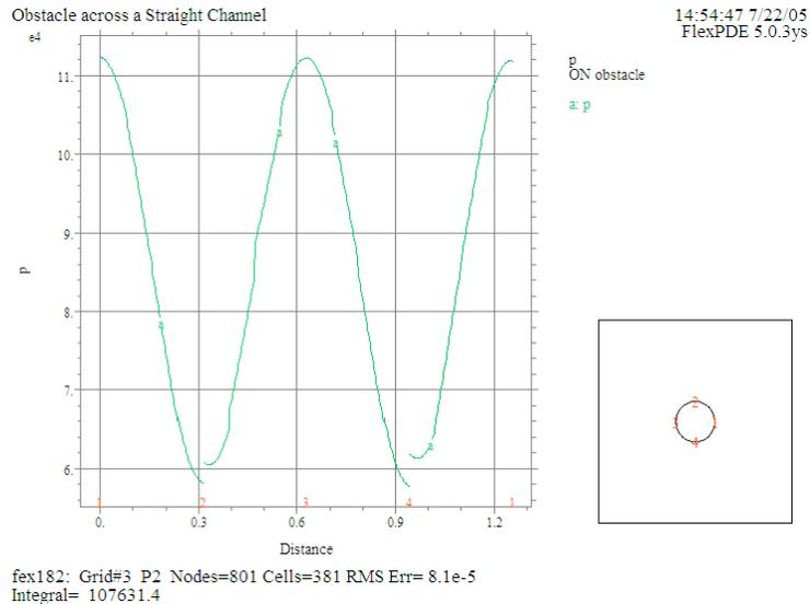
To the left and also to the right of the obstacle (points 1 and 3), we find pressure values larger than the ambient value ( $1e5$ ). We could
