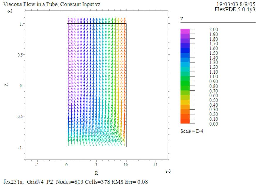
The three elevation plots demonstrate the constancy of the flux along the tube. The last plot (below) indicates that the derivative of  $v_z$  is linear, i.e. that the velocity profile has become parabolic.
