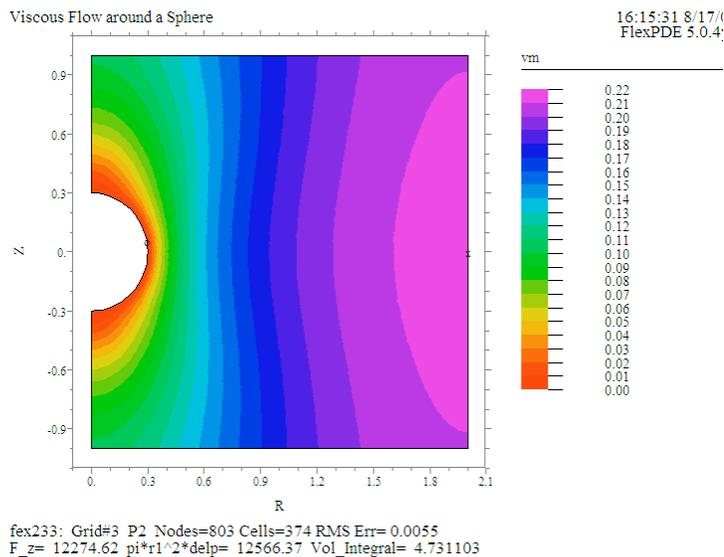
We have included a comparison with the force due to the driving pressure, which evidently is 2.4% higher than the value obtained by integration.
