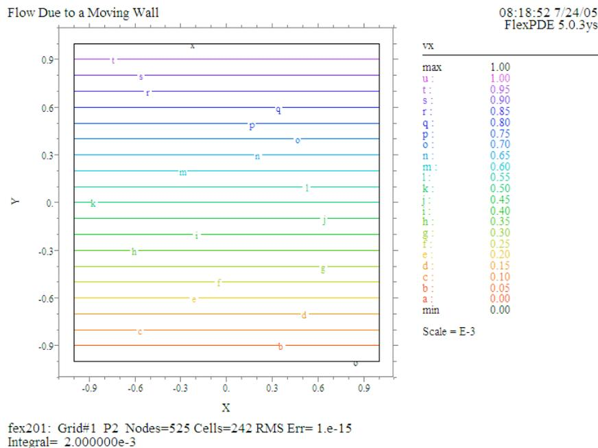
The plot below suggests that  $\nabla \cdot \mathbf{v}$  vanish everywhere. Applying the integral definition of the divergence (pp.21,23) to a small box parallel to the axes, we find that only the sides perpendicular to the x-axis contribute, and with opposite signs. The plot of div(v) does not yield exactly zero, but the contours are irregular and the values are small compared to an estimate of the maximum possible derivative,  $\delta v_x / \delta y \cong 10^{-3}$ .
