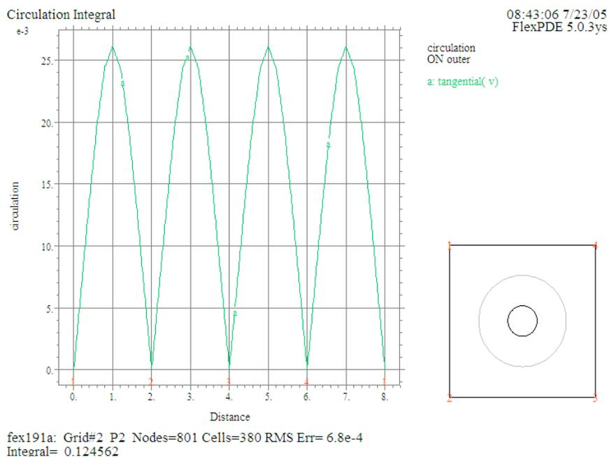
We now calculate the circulation over three different curves, all enclosing the region where  $\omega$  is non-zero. The above plot shows the tangential velocity-component on the square boundary. We find the other two integral values to be about the same.
