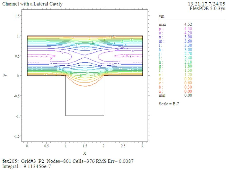
Both vector plots demonstrate that circulation occurs in the cavity, and the *curl* is again non-zero. The plot below clearly shows the center of circulation.
