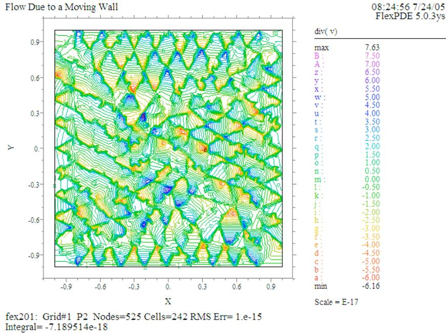
Using the line integral definition of *curl* (p.21), we first notice that its value must be the same everywhere. The local *curl* must thus equal the average value we obtain from a line integral along the boundary, which amounts to  $(0 - v_{x0}2L_x) / (2L_x \cdot 2L_y) = -v_{x0}/2 = -5e - 4$ . This result is borne out by the plot of  $\text{curl}(v)$ .
