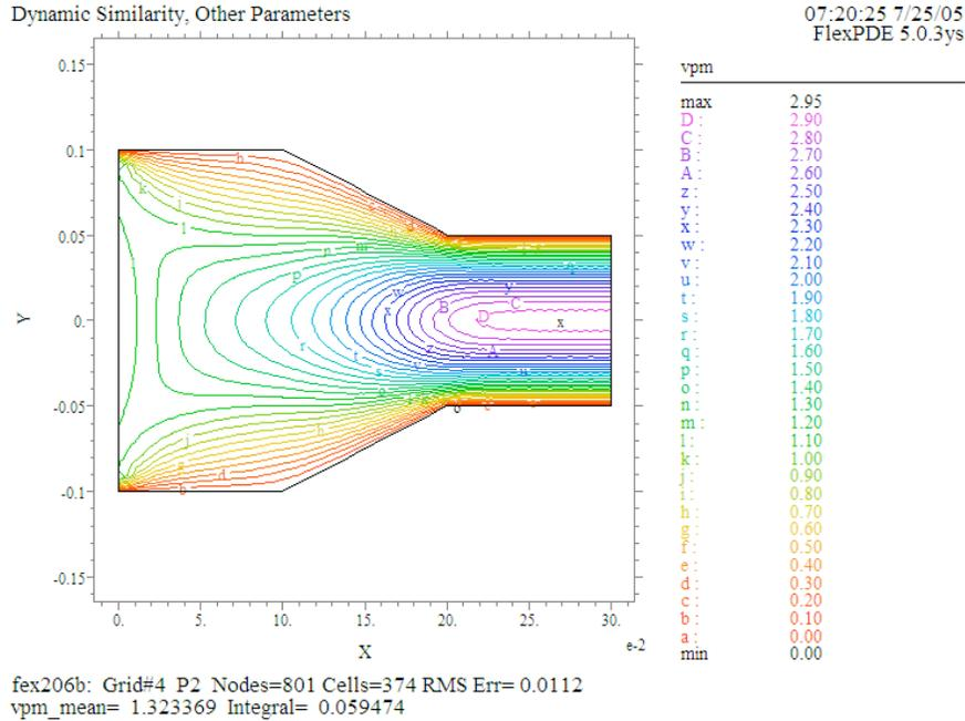
From the third plot it appears that  $pp$  varies over the same range in the two descriptors. In order to make a more accurate comparison, we could integrate the results. Considering that the geometrical sizes are different (by a factor of 100), we should also divide by the area to obtain mean values. These also turn out to be nearly equal.
