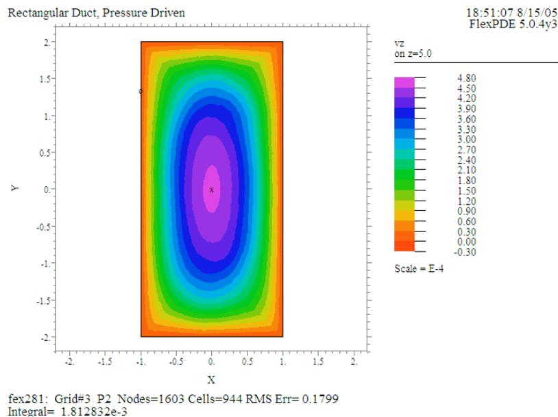
The last elevation plot shows that the actual velocity is about 10% lower than the analytical result for the channel (p.259). In the latter case, however, the larger side is infinite and hence the drag forces from the two distant walls are absent.
