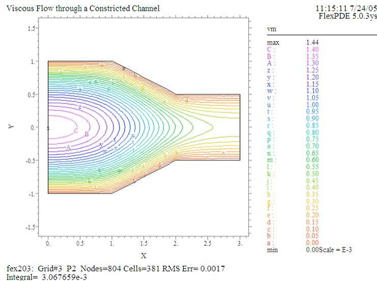
The next plot shows that the divergence definitely is non-zero. We also obtain a similar indication from the two elevation plots. The integral value reported on the bottom line is obviously equal to the volume of liquid transported through the cross-section (per second and meter of depth in  $z$ ). The two integral values show that the fluxes
