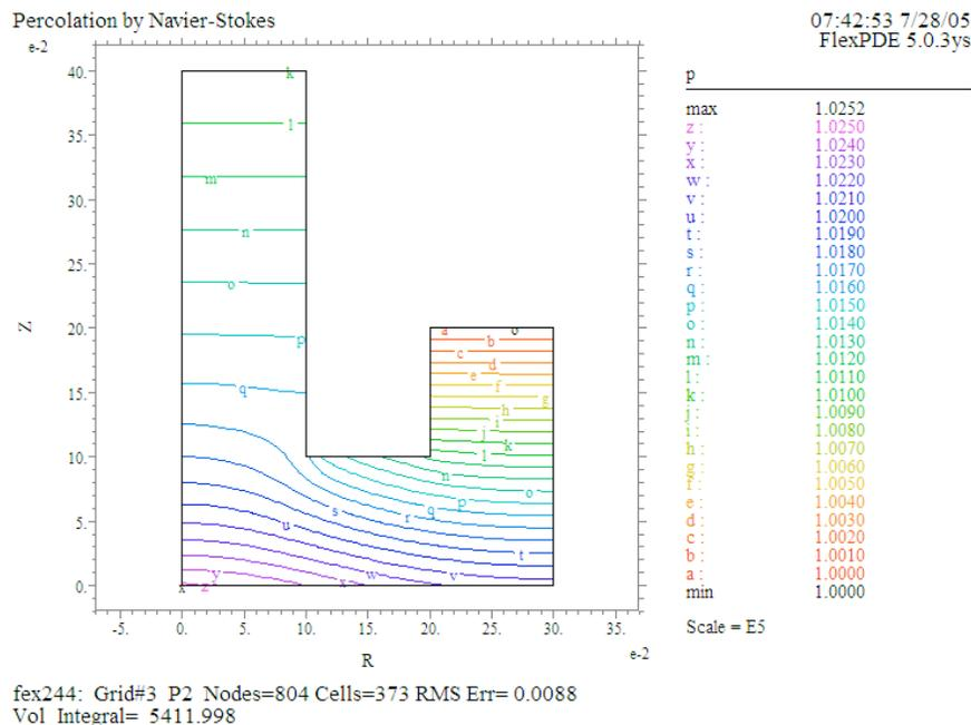
We may again compare the two formalisms by putting  $F_{gz}=0$  in the *definitions* section. The contour plots of pressure then become very similar. The vector plots of the velocity are also much the same as before. A sensitive test is to compare the plots of  $v_m$ , where we note that the volume integral now is  $4.789e-8$  against  $4.820e-8$  in *fex243*. The agreement is remarkable, considering that the PDEs and the boundary conditions are different.
