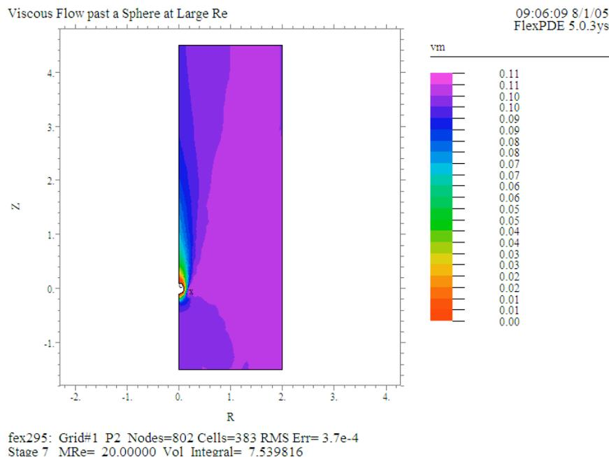
Because of the poor pressure data, the drag force differs considerably from the Stokes expression at the smallest values of  $MRe$ , the integrated ratio  $p/drag\_S$  being as small as 0.13 in the first stage. Above stage 3, however, it is still possible to recognize the variation versus  $MRe$  that we recorded before.
