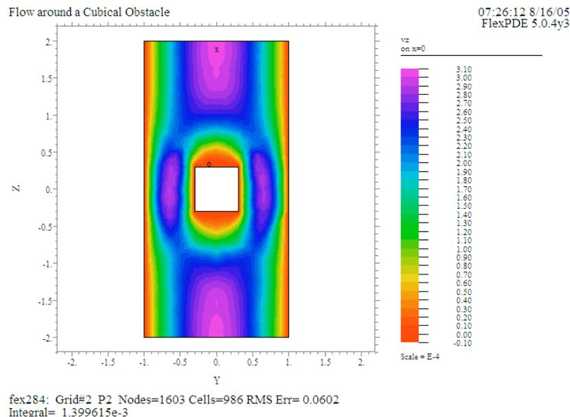
The next figure shows the direction of flow in the region close to the cube. It confirms that the speed vanishes on all the faces of the cube.
