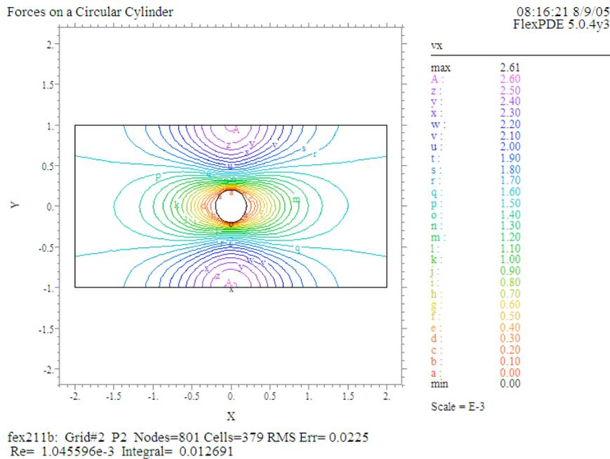
The drag force reported in the table below is  $F_x=194.2$ , while we obtain  $\text{delp} \cdot 2 \cdot L_y = 200$  for the same force from the applied pressure, the difference being about 3%. The viscous force on the wall ( $F_{\text{wall}_x}$ ) is evidently negligible. Using the Professional Version we again obtain much better agreement.
