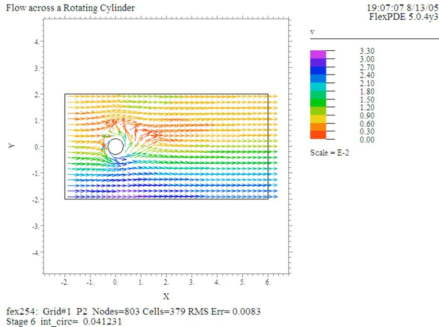
Since the liquid slips over the walls, the horizontal force  $f_x$  on the cylinder (per unit length) must be closely equal to the driving force on the liquid at the left end. For the final stage we thus have  $f_x = 2 * Ly * delp = 0.12$ .
