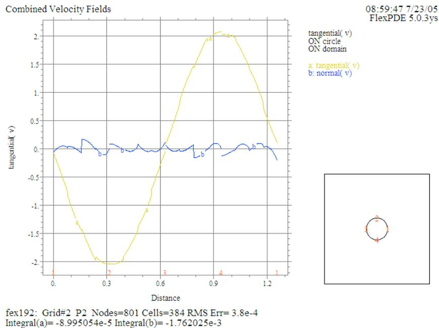
The above plot shows that  $v_n$  is in fact smaller than  $v_t$  but fluctuates noticeably around zero. This is the best that can be done, however, with this limited number of nodes. Using the Professional Version with a smaller value of `errlim` we obtain less scatter and no visible net variation.
