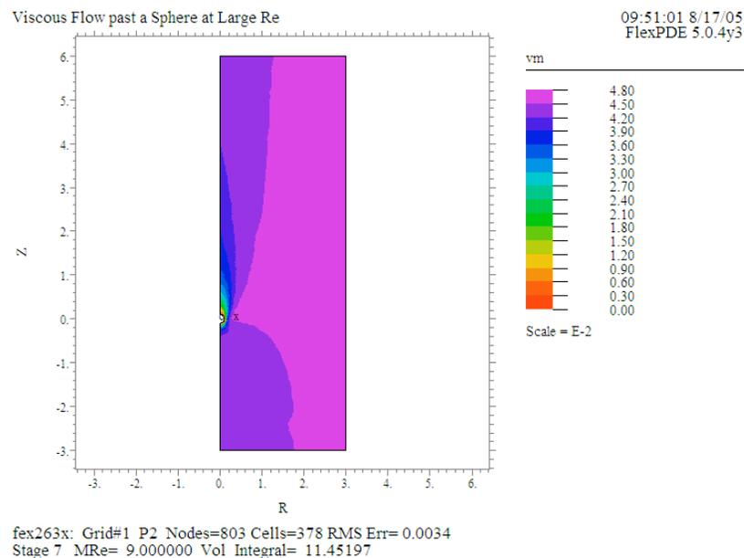
The above contour plot of  $vm$  shows the speed distribution in the last stage of the calculation. The low-speed region extends far toward the exit.
