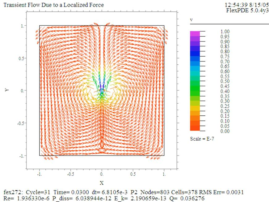
In the *definitions* segment we prepared to calculate the total kinetic energy (per unit depth of the domain), and also the total power of viscous dissipation ( $P_{diss}$ , p.285). We have combined these to form a ratio  $Q$ , analogous to the quality of a resonant cavity.
