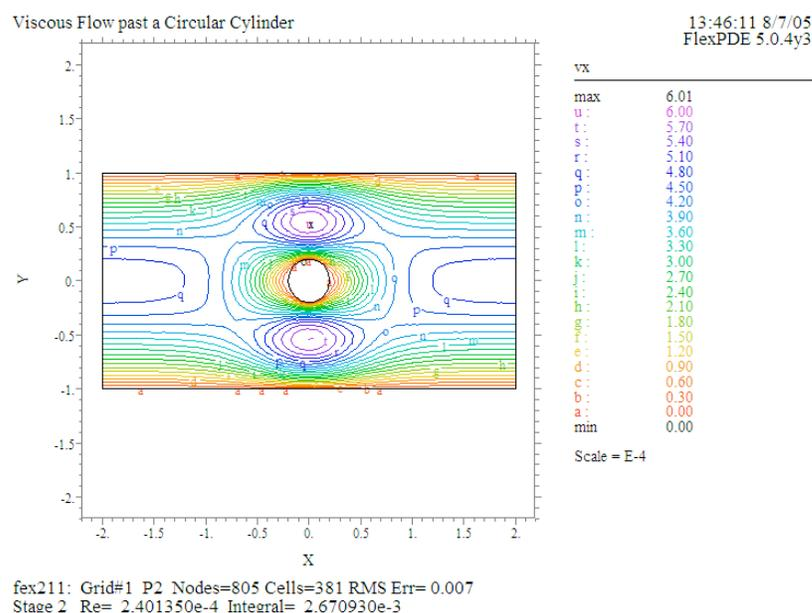
Switching between stages 1 and 2 we find no visible change of the contours of  $v_x$ , and the integral values differ only in the fourth decimal. The variation is about as small for  $v_m$  and  $p$ . For the rest of the examples in this chapter we shall thus replace  $natp$  by 0 on the basis of experience.
