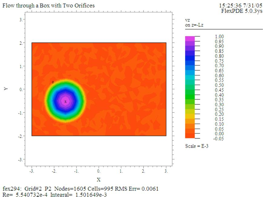
The next plot shows the flow in a plane going through the centers of both the entrance and the exit. The symmetry is evident.
