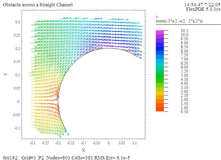
The plot also illustrates the phenomenon of stagnation. The color serves to indicate the magnitude. Here, the speed vanishes at  $y = 0$  on a line perpendicular to the figure.
