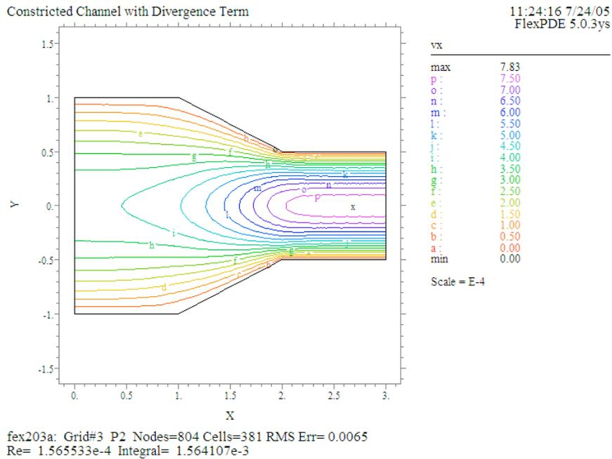
The elevation plots across the channel both exhibit parabolic velocity profiles (below). They also demonstrate the conservation of mass and volume, because we find the two flux integral values to agree within 0.02%.
