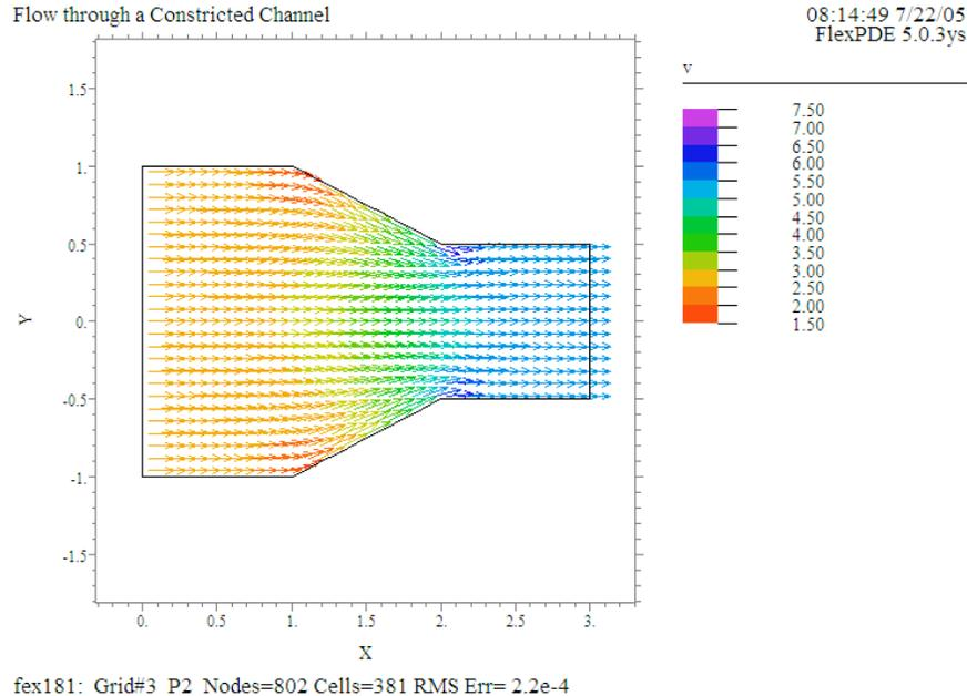
We also see from the plot of  $v_m$  (not shown here) that the speed increases by a factor of about two from input to output, i.e. in inverse proportion to the channel width. This is of course in accord with the conservation of mass and volume, a principle that was incorporated into the PDE by the vanishing divergence. Notice, however, that we did not explicitly introduce this constancy in the boundary conditions at the ends, although we could well have done so.
