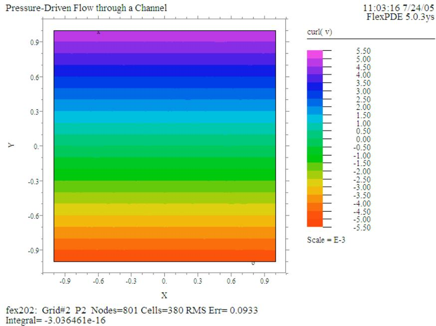
We may also calculate the vorticity from the analytic solution as  $-\partial v_x / \partial y$ . This is another example of innocent-looking, laminar flow that proves to be rotational.
