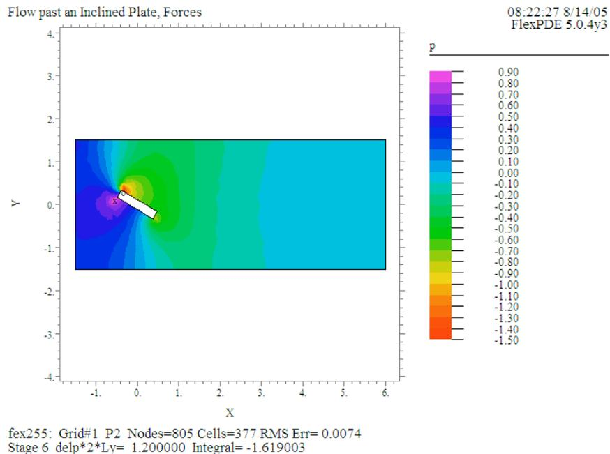
From the combined integral in the elevation plot (below) we obtain the lift force. For  $MRe \approx 62$  it becomes 0.67, or only 56% of the drag.
