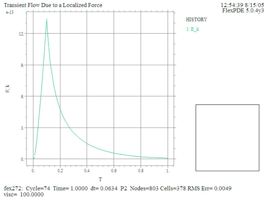
The above figure is a history plot displaying the variation of the kinetic energy versus time. Evidently, the accumulated energy increases steadily while the force is on, but after the latter is reduced to zero it gradually decreases. This obviously means that the residual motion of the fluid for  $t > 0.1$  dissipates the kinetic energy stored.
