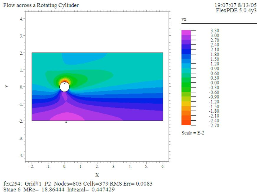
In the above plot for the highest pressure, we notice that the region of small speed, which was symmetrical for small  $MRe$ , now has shifted downstream.
