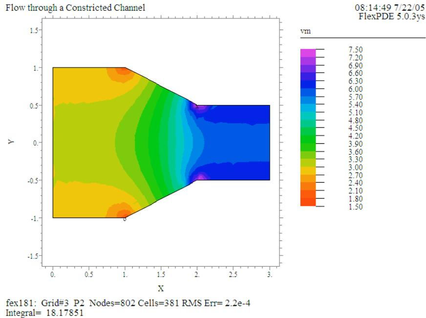
In the *definitions* segment we declared the vorticity  $\omega$  to be a variable, but we waited until *boundaries* to assign values to it. The plot of  $\text{div}(v)$  shows the result to be zero in the liquid, and the next plot suggests that  $\text{curl}(v)$  also vanishes, as required.
