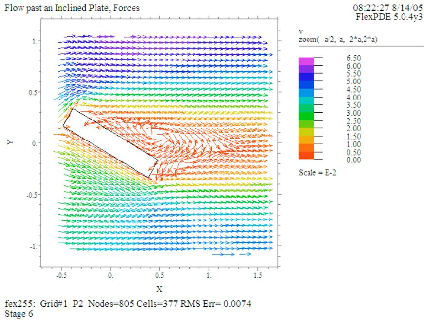
The plot below demonstrates that the pressure at large MRe becomes higher under the airfoil, which partly explains the lift force. The plot also reports the force on the liquid domain, which should be equal to the *drag* force on the slab.
