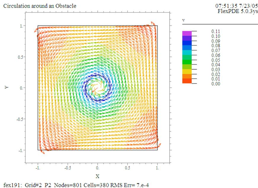
According to the above plot, the velocity on the outer boundary is parallel to the border. The first elevation plot, comparing the normal and tangential components of  $v$  confirms this fact.
