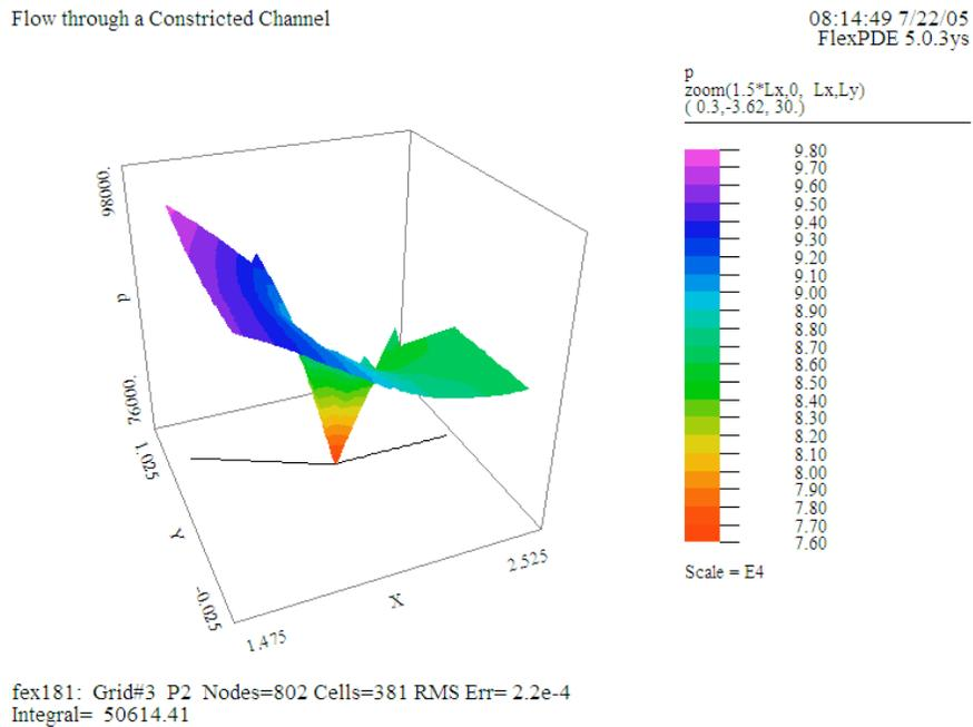
From the above surface plot of  $p$  it is evident that the pressure has a minimum at the corner where the speed peaks. The color code
