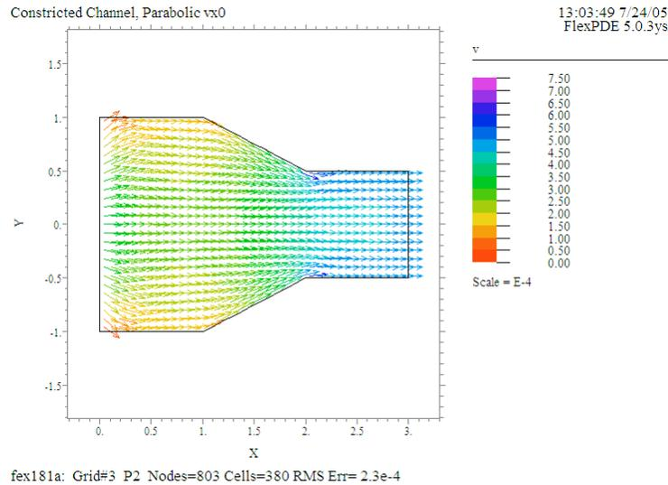
This example shows that the behavior of viscous flow is dramatically different from that of potential flow. It is possible, however, to consider viscous flow through a channel as potential flow in a region sufficiently far from the walls. The region close to the wall, where the vorticity is large (the boundary layer), may be treated separately.
