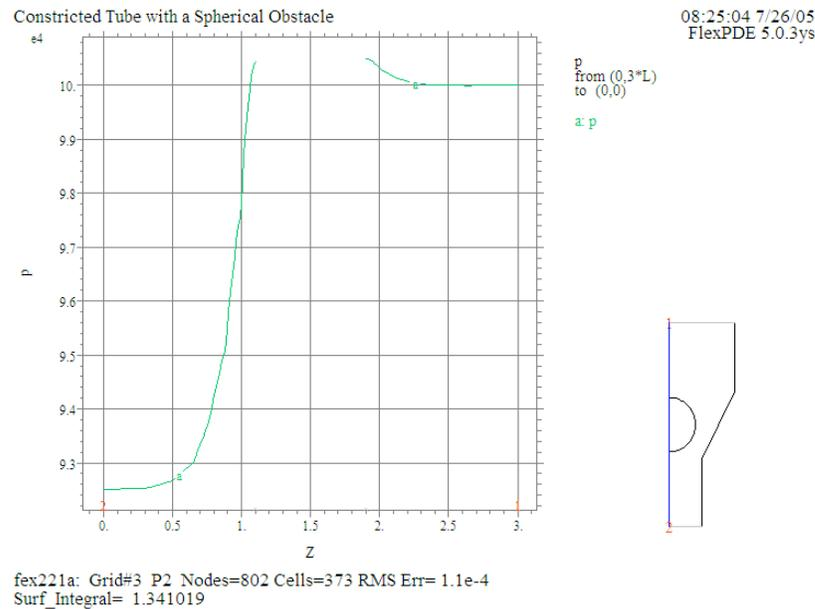
It may be surprising to discover that the gain in kinetic energy per unit time from input to output is closely the same as without the obstacle.
