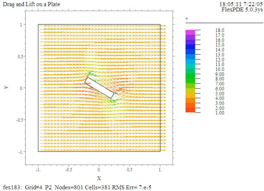
Although the pressure distribution below seems to be symmetric with respect to the coordinate axes, this is less obvious than in the preceding example. It is clear, on the other hand, that the stream exerts a torque on the plate.
