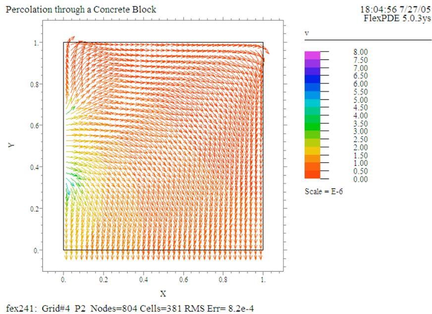
Although this plot looks plausible, we did not include the force of gravitation, which is of appreciable magnitude in this problem. In fact, there is no obvious way of including any volume force in these equations.
