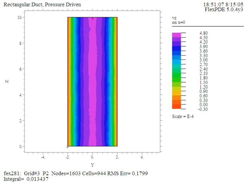
The figure below illustrates that the longitudinal velocity component  $v_z$  vanishes on the other walls, as required. The integral value gives us the flux through the cross-section. Comparing the three corresponding plots we find that the flux values are closely the same, which confirms that mass is conserved.
