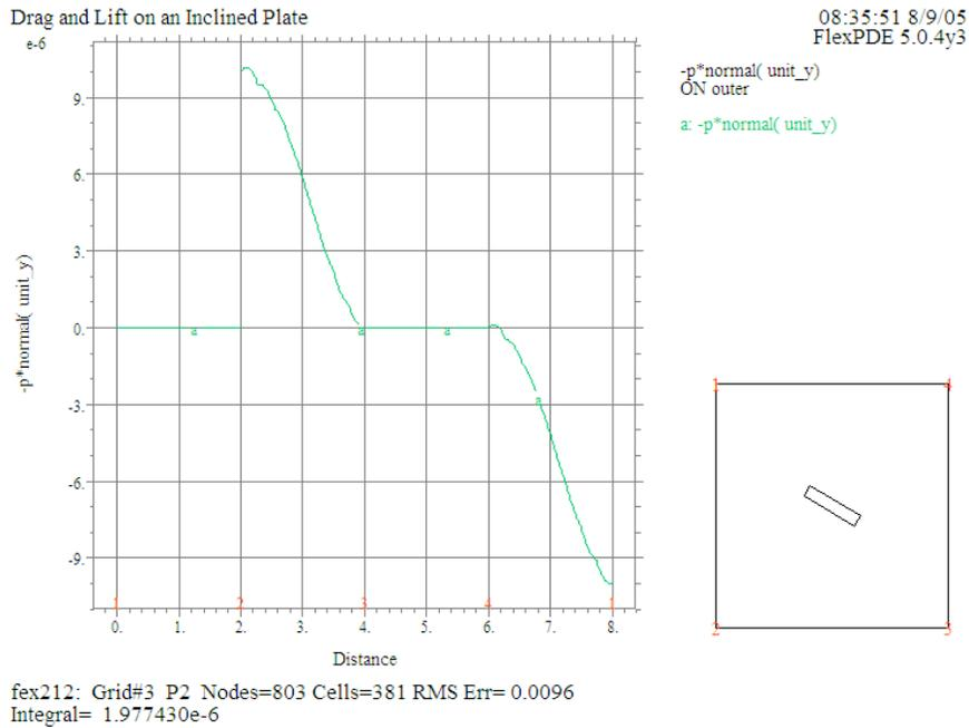
We have thus found that the combined force from both walls is small compared to the force ( $2.0 \cdot \Delta p = 2e-5$ ) applied by the driving pressure. The lift force is only about 10% of the drag force on the plate, which demonstrates that an airplane does not fly well at small speed in a highly viscous medium.
