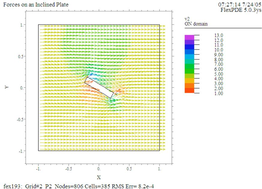
The following plot of  $v_t$  and  $v_n$  illustrates that the normal component is relatively small on the long sides, but that the few node points on the short sides do not yield the ideal zero, but positive and negative slopes.
