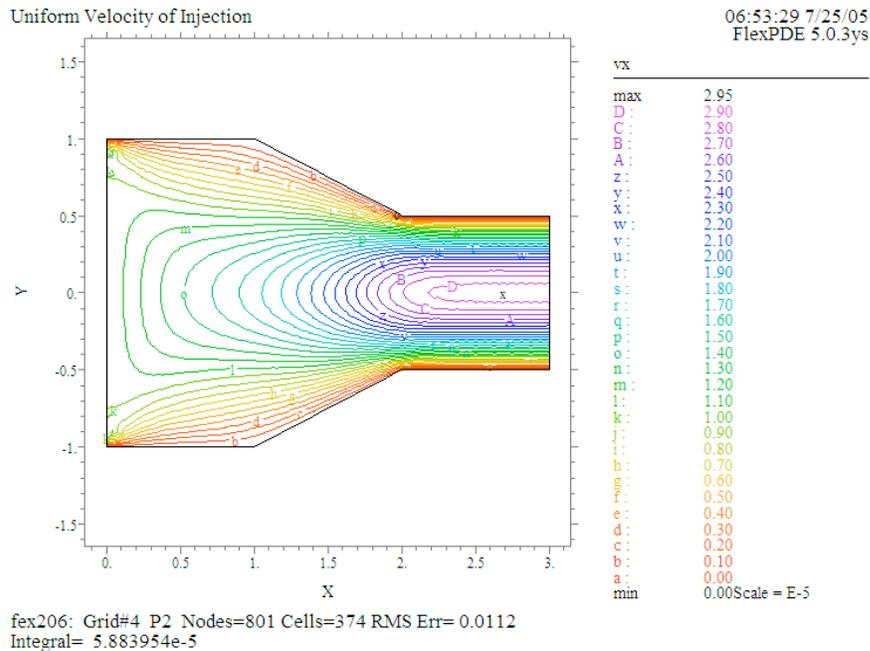
The elevation plots of  $v_x$  across the ends show in more detail how the initially uniform profile modifies into a parabolic one, as is clearly confirmed by the derivative. Obviously, the velocity component  $v_x$  is not strictly uniform over the input, but that is caused by the discontinuity at the walls. The integrals confirm that flux is conserved.
