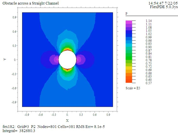
The elevation plot below presents the pressure variation on the surface of the obstacle. The left-right symmetry, as well as the up-down symmetry, is clearly evident from this figure.
