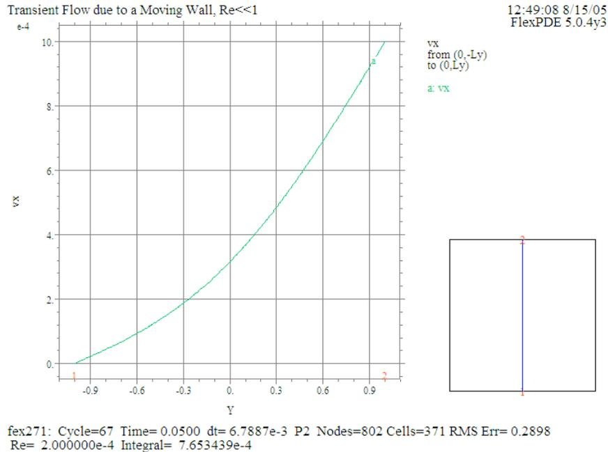
There is an analytic solution<sup>9p191</sup> in terms of Fourier series that could be used for comparison. At large times we would expect to recover the linear result from *fex201*.
