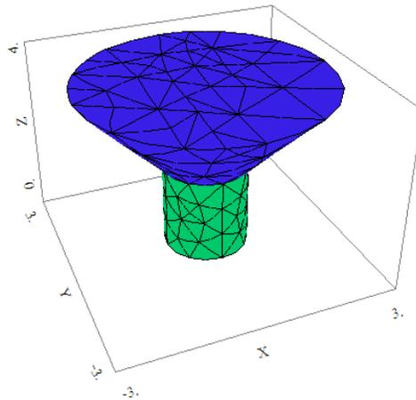
We create the region 'domain' by extruding a circle with radius  $r_1$ , starting from the base plane, i.e.  $z=0$ . Thus, we initially obtain a volume limited by the planes '1' and '3' and a circular cylinder. It remains to *exclude* the parts outside the cone and the smaller cylinder below.
