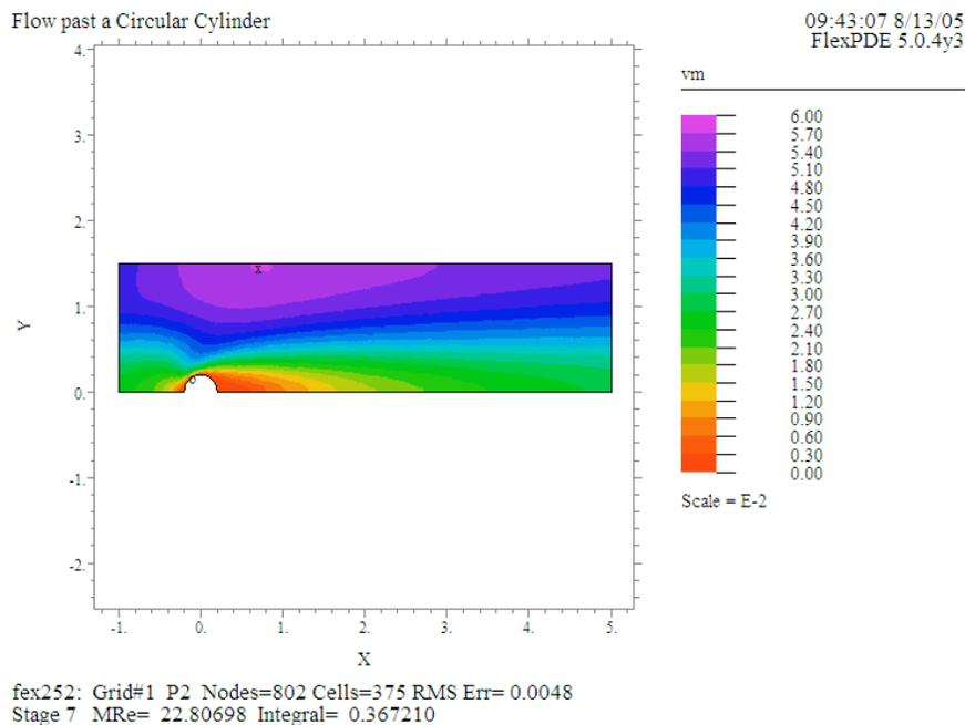
The above plot shows the speed  $v_m$  at  $MRe \approx 23$ . The left-right symmetry we found at small  $MRe$  (p.278) is evidently broken. There is now an extended region in the wake of the cylindrical obstacle where the speed is very small.
