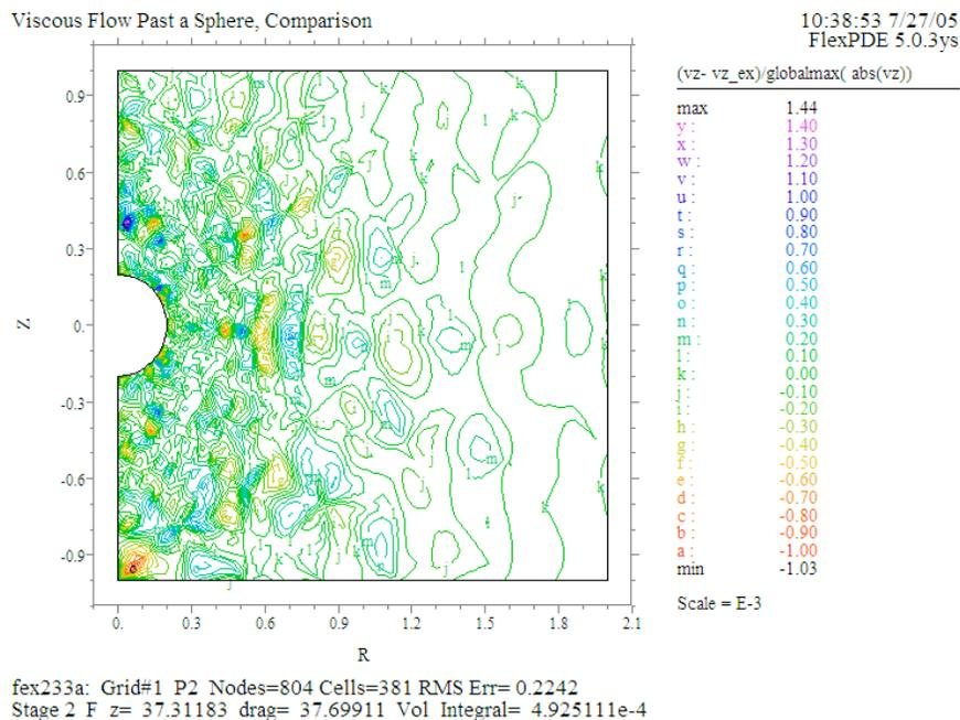
The above plot shows that the maximum relative error in the case of  $v_z$  is about 0.1%, but the largest values occur in a small region of the domain. The agreement is roughly 1% for  $v_r$  and  $p$ .
