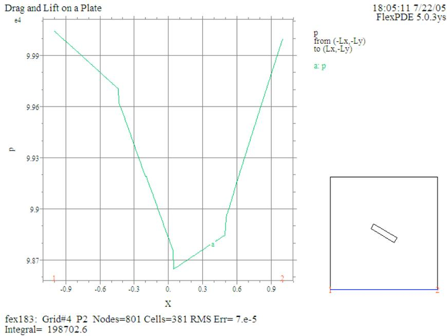
Taking the difference of the force integrals we find the value  $-7.7$  for the  $x$ -component and  $-0.1$  for the  $y$ -component. We compare these forces to an estimate (brute\_force) of that acting on the surface facing the stream, i.e.  $p_0 \cdot 2 \cdot y^2$ . We find that the force components are smaller than the reference value by a factor of at least 4000.
