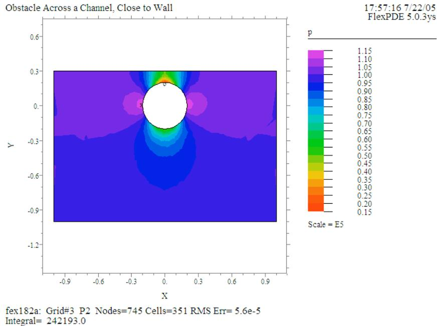
Evidently, the pressure pushes the obstacle toward the nearby wall. This effect is vaguely analogous to the suction felt when you stand close to a passing train.
