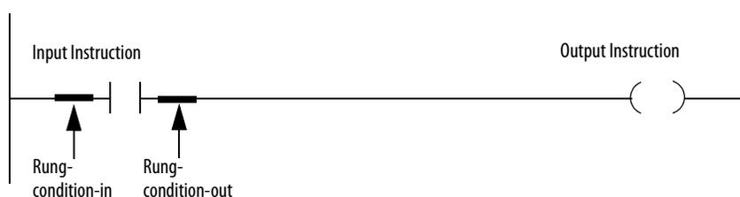
If the rung-condition-in to an input instruction is true, the controller evaluates the instruction and sets the rung-condition-out based on the results of the instruction. If the instruction evaluates to true, the rung-condition-out is true; if the instruction evaluates to false, the rung-condition-out is false.
