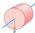
(g) Thin-walled hollow cylinder
