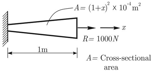
**Fig. 5.5.** Bar problem with varying bar cross-sectional area
