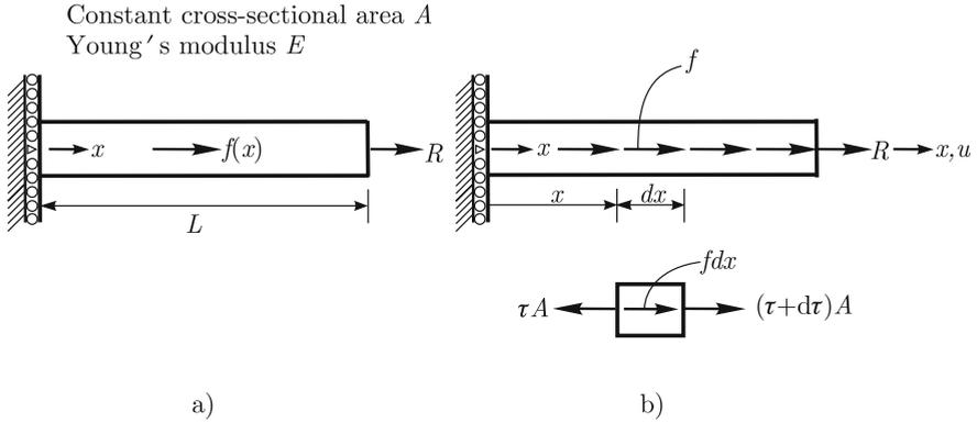
**Fig. 5.1.** a) Bar problem; b) Differential equilibrium for bar problem (plane sections remain plane)
