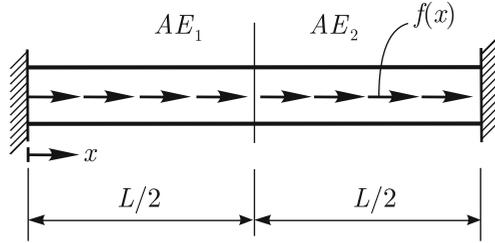
**Fig. 5.6.** Bar problem with varying material properties
