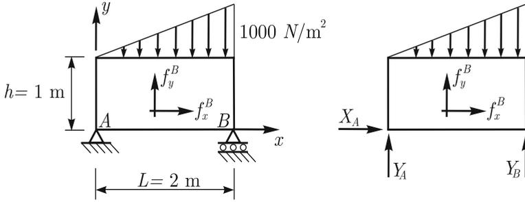
**Fig. 5.7.** a) Definition of the plane stress problem,  $f_x^B = 0$ ,  $f_y^B = -2400 \text{ N/m}^3$ ,  $t = 0.1 \text{ m}$  (thickness); b) Equilibrium of the plate including reactions
