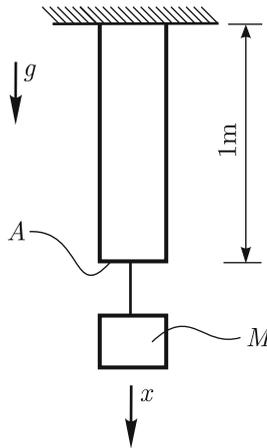
**Fig. 5.4.** Steel bar subjected to gravity. The density  $\rho[\text{kg}/\text{m}^3]$ , the area  $A[\text{m}^2]$  and the mass  $M[\text{kg}]$
