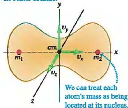
**(b) Rotational motion.** The molecule rotates about its center of mass. This molecule has two independent axes of rotation.
