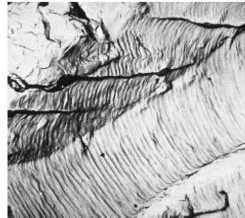
**FIGURE 9.31** Transmission electron fractograph showing fatigue striations in aluminum. Magnification unknown. (From V. J. Colangelo and F. A. Heiser, *Analysis of Metallurgical Failures*, 2nd edition. Copyright © 1987 by John Wiley & Sons, New York. Reprinted by permission of John Wiley & Sons, Inc.)
