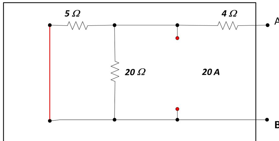
$$R_{TH} = R_N = 4\Omega + (5\Omega // 20\Omega)$$
