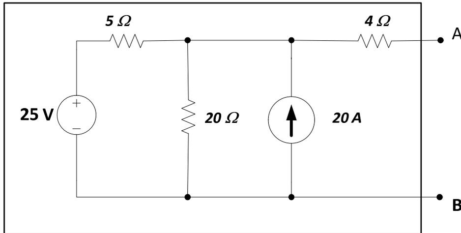
ANULA-SE AS FONTES E DETERMINA-SE A RESISTÊNCIA EQUIVALENTE VISTA DOS TERMINAIS DE INTERESSE.
