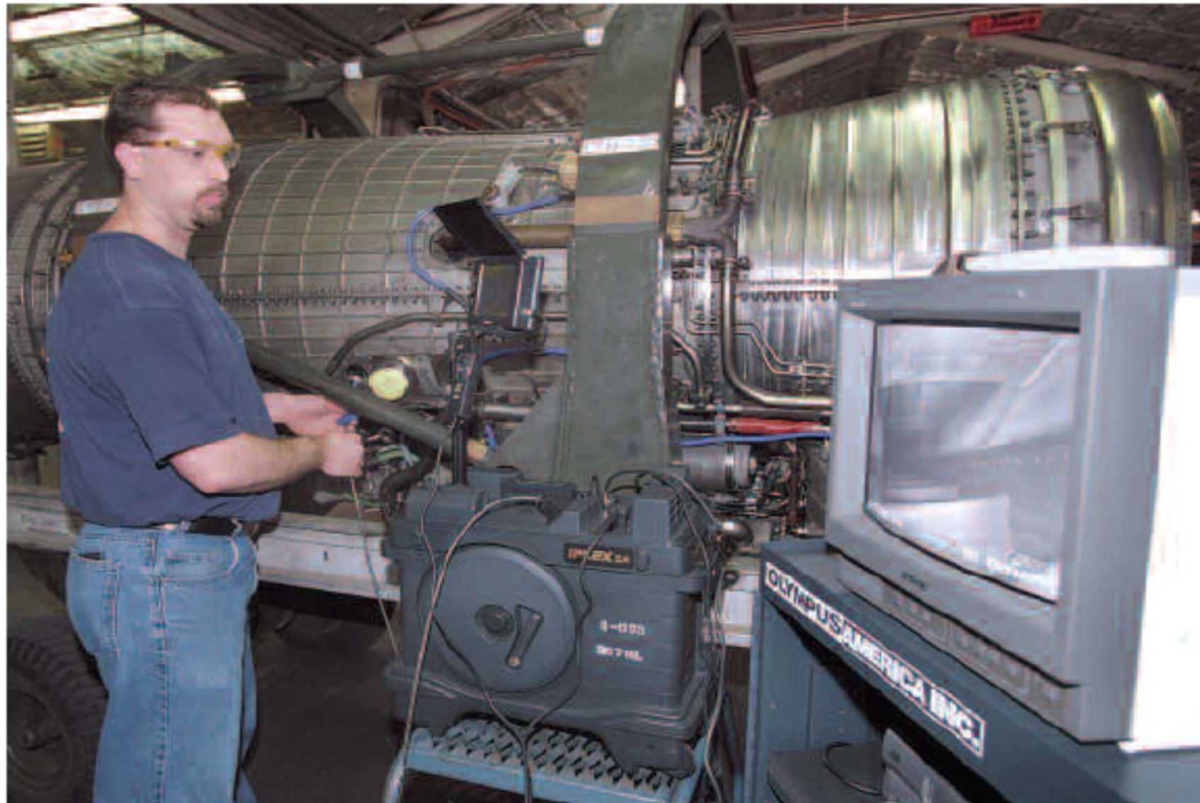
Figure 2. An Inspector at Tinker Air Force Base Gets a Magnified View of an Engine's High-Pressure Turbine Area with a New Digital Fiber-Optic Borescope. (Photo Courtesy of US Air Force; Photo taken by Margo Wright)
