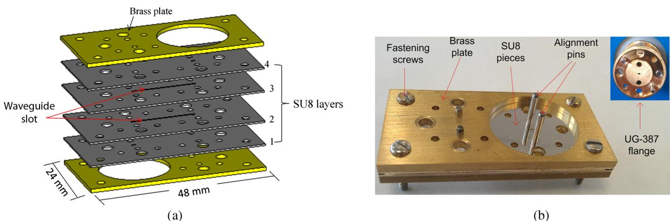
**Fig. 6** Typical integration structure of passive terahertz devices: (a) schematic assembly configuration and (b) an example of assembled 300 GHz waveguide.<sup>10</sup>
