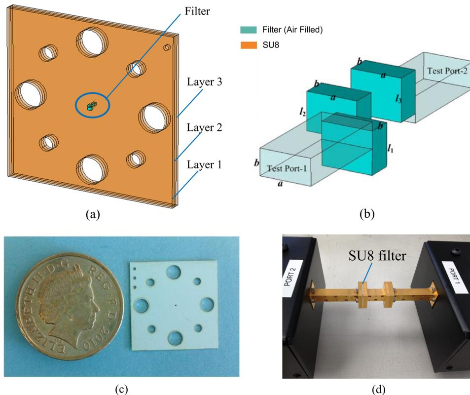
**Fig. 2** A WR-1.5 band filter made by SU8 process.<sup>9</sup> (a) Configuration of the whole filter comprising of three layers with the same thickness of 191  $\mu\text{m}$ . The outstanding part stands for the filter; (b) the filter structure; (c) one SU8 layer with silver coating; (d) the measurement setup. The filter (based on three SU8 shims) is sandwiched between two waveguide flanges of measurement equipment.
