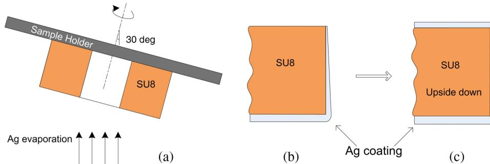
**Fig. 5** Schematics of metallizing the sidewall of SU8 components through evaporation: (a) configuration of the SU8 components in the evaporation chamber; (b) silver thickness distribution after coating on one side; and (c) full coverage of sidewall with silver after evaporation on both sides.
