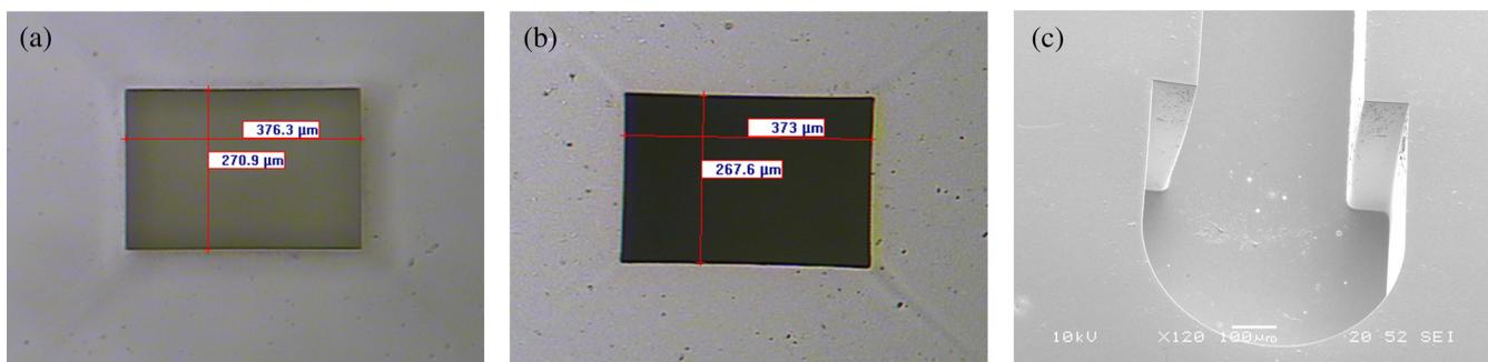
Fig. 7 Measurement of SU8 pieces at different stages of the fabrication process: (a) after development; (b) after metallization; and (c) metallization quality and double-layer integrity inspection in scanning electron microscope.
