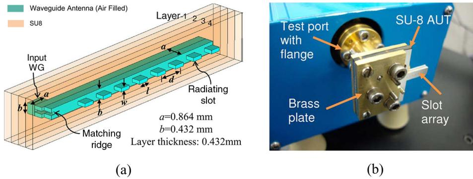
**Fig. 1** A WR-3 band antenna.<sup>18</sup> (a) The 300-GHz slotted waveguide antenna with the port flange of the test equipment. (b) Enlarged view of the slot array and the H-plane bend formed of four layers. (The outstanding structure in the central areas represents the hollow channel and slots.)
