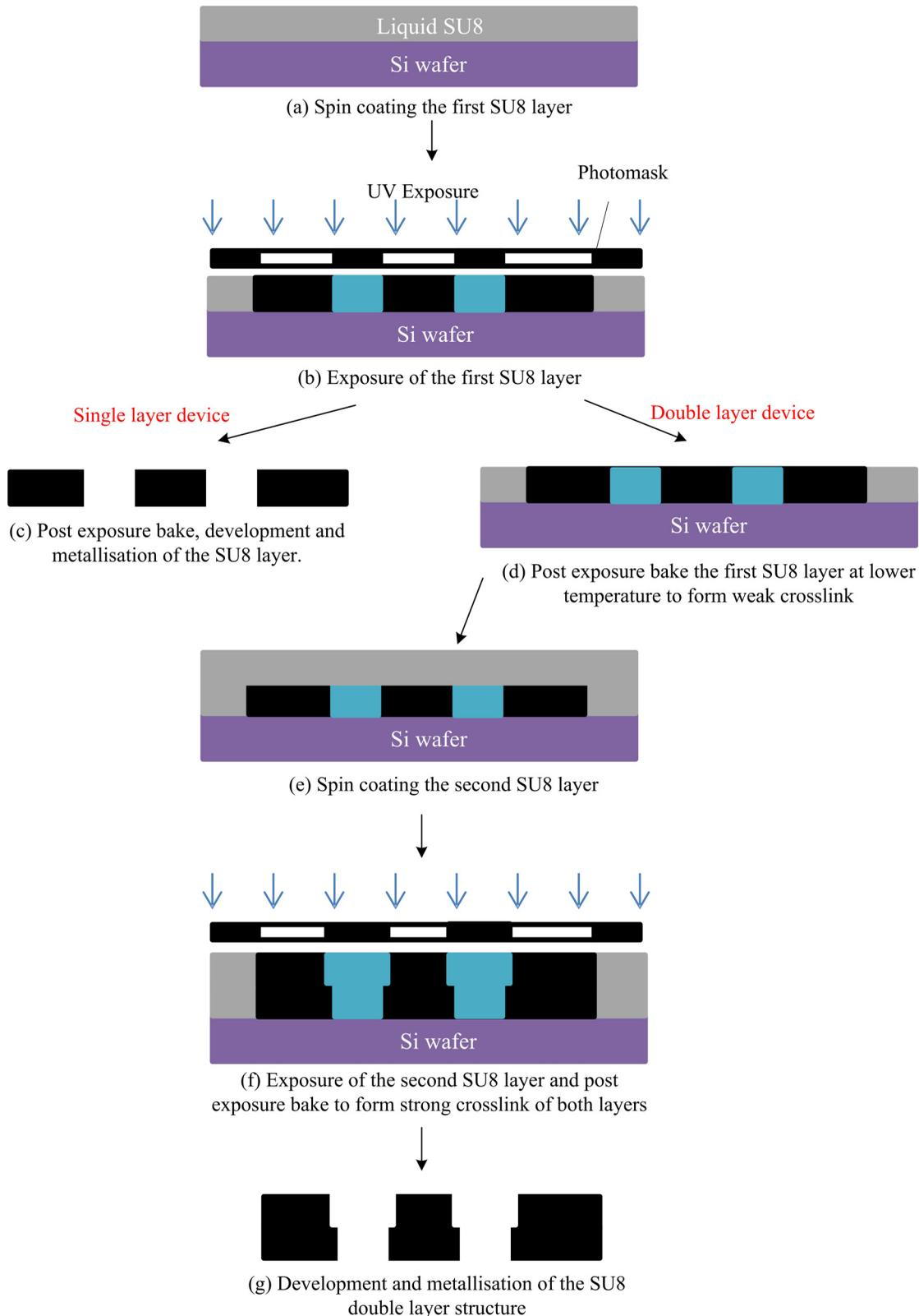
**Fig. 4** Typical SU8 fabrication process flow.
