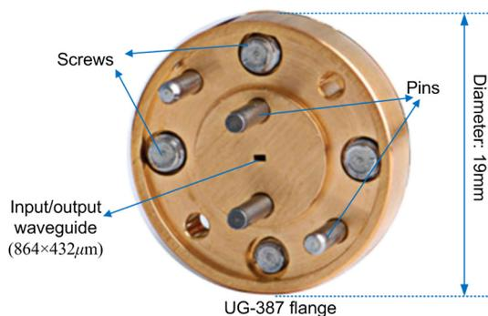
**Fig. 3** A UG-387 flange that has been used widely by terahertz (THz) waveguides.
