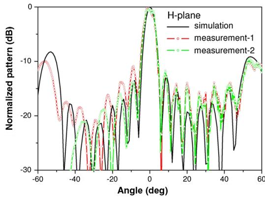
Fig. 9 Measurement results of the WR-3 antenna,<sup>18</sup> measured H-plane radiation patterns in comparison to simulations.
