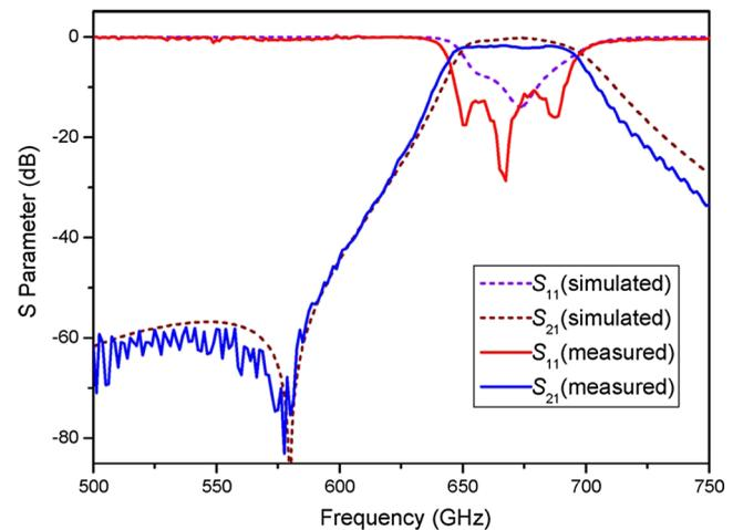
Fig. 8 Measurement results of the WR-1.5 band filter made from SU8.<sup>9</sup>
