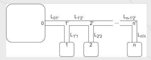
$$\begin{cases} \frac{\partial P_i}{\partial t} = \frac{(P_{i'} - P_i)}{CiR_{i'-i}} \\ P_{i'} - P_i = \dot{m}_i R_{i'-i} \\ \frac{\partial P_{i'}}{\partial t} = \dot{m}_{i'} \frac{RT}{Vi'} = \frac{\dot{m}_{i'}}{C_{i'}} \\ P_{i'-1} - P_{i'} = \left(\sum_{j=i}^n \dot{m}_i + \dot{m}_{i'}\right) R_{(i-1)'-i'} \end{cases}$$
