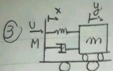
$$\begin{aligned} \cdot m_1 \ddot{x} = k(x - y) + b(\dot{x} - \dot{y}) &\Rightarrow \ddot{y} = \frac{k}{m}x - \frac{k}{m}y + \frac{b}{m}\dot{x} - \frac{b}{m}\dot{y} \\ \cdot M\ddot{x} = U - k(x - y) - b(\dot{x} - \dot{y}) &\Rightarrow \ddot{x} = \frac{U}{M} - \frac{k}{M}x + \frac{k}{M}y - \frac{b}{M}\dot{x} + \frac{b}{M}\dot{y} \end{aligned}$$
