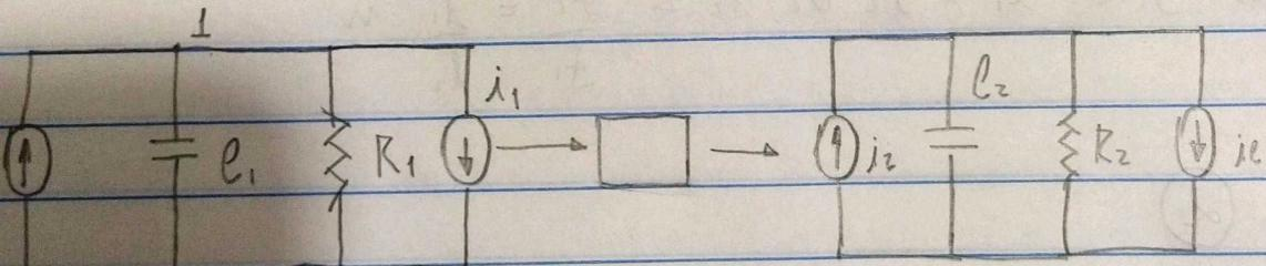
$$\text{nó 1: } i_n - V_1 \left( C_1 D + \frac{1}{R_1} \right) = i_1 \Rightarrow J_1 \cdot \ddot{\theta}_1 + B_1 \cdot \dot{\theta}_1 = T_m - T_1$$
