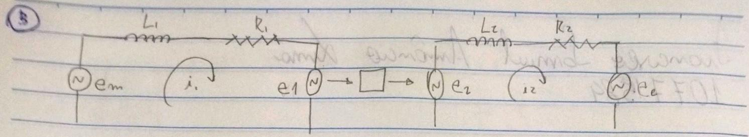
$$\text{mola } i_1: e_m = e_1 + i_1(L_1 D + R_1) = 0 \Rightarrow J_1 \ddot{\theta}_1 + B_1 \dot{\theta}_1 = T_m - T_1$$
