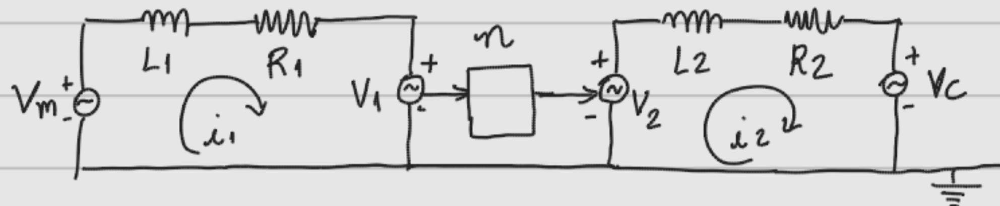
$$V_m - i_1 (L_1 D + R_1) - V_1 = 0 \Rightarrow J_1 \ddot{\omega}_1 + B_1 \omega_1 + T_1 = T_m$$
