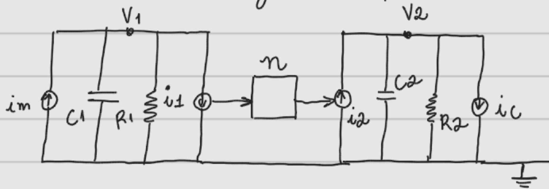
$$i_m - V_1 \left( C_1 D + \frac{1}{R_1} \right) - i_1 = 0 \Rightarrow J_1 \ddot{\omega}_1 + B_1 \omega_1 + T_1 = T_m$$
