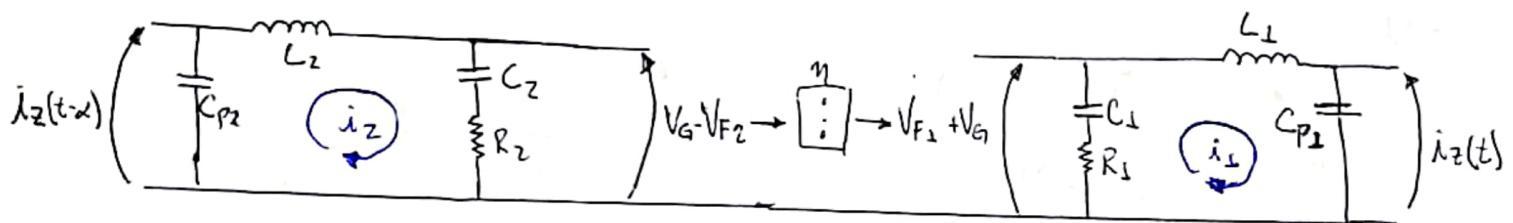
$$\text{Malha 1: } i_1 \left( L_1 D + R_1 + \frac{1}{C_1 D} + \frac{1}{C_{p1} D} \right) - i_2(t) \left( \frac{1}{C_{p1} D} \right) = V_{F1} - V_G$$
