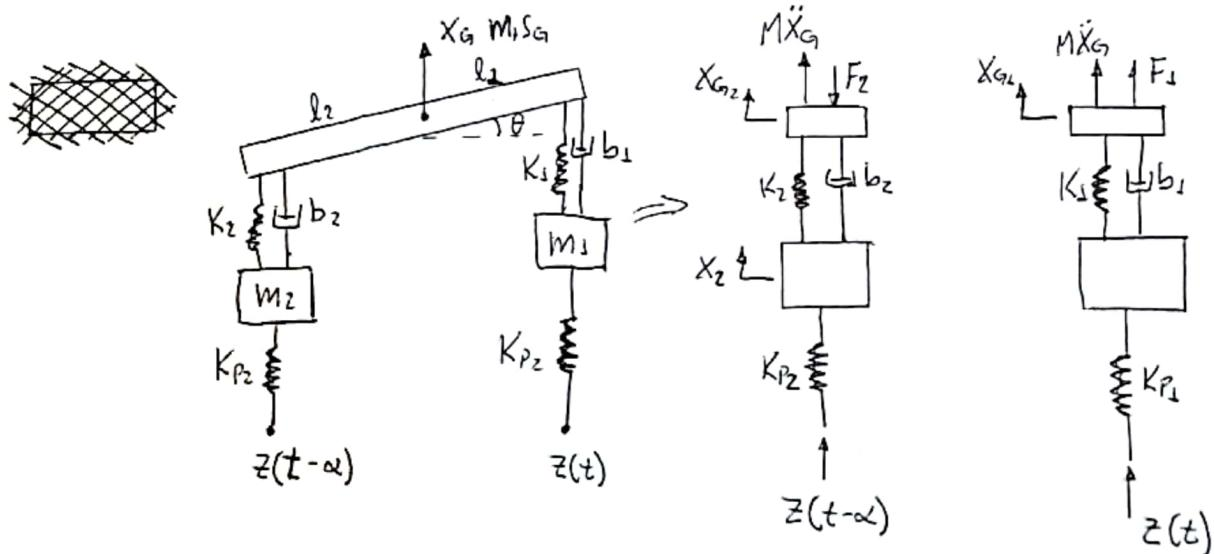
$$\eta = \frac{l_2}{l_1} \quad F_2 l_2 = F_1 l_1 \rightarrow \eta = \frac{F_1}{F_2}$$
